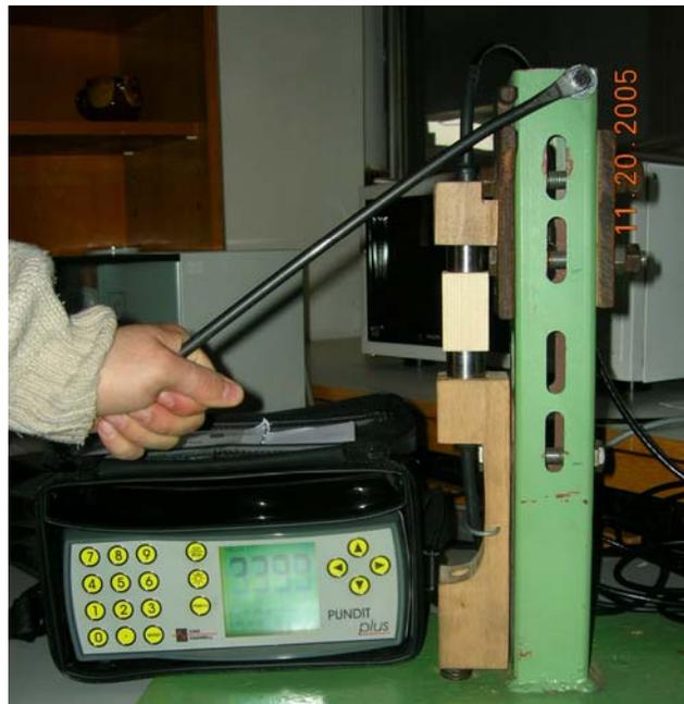
**Fig. 1.** Measurement of the UW velocity in the longitudinal direction of a spruce specimen using constant pressure on the transducers mounted in a wooden-metal stand
