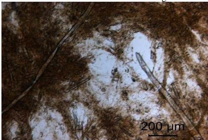
Fig. 4. Light microscope image of a foam fraction after flotation of TMP water with 150 ppm chitosan and 40 ppm SDS
