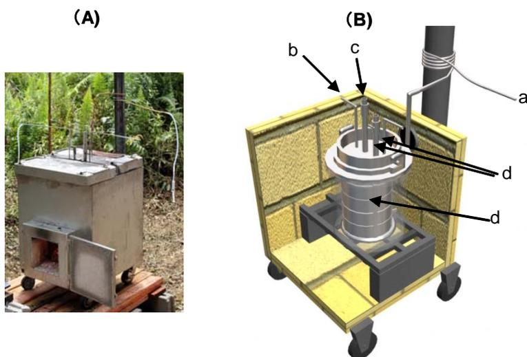
**Figure 1.** Real Image (A) and drawing image (B) of electric-free furnace for AC production. a, water inlet connected to bottom; b, water inlet connected to top; c, thermocouple tube; d, gas outlet; e, four layers of sample baskets.
