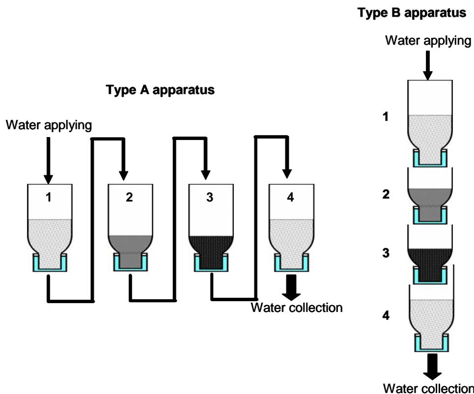
**Figure 2.** A mobile water-purification apparatus. In Type A, the purification was carried out stepwisely through 4 layers, and in Type B, layers of purification agents are directly connected. 1, Keranggas as first layer (15 g and 25 g); 2, Wood charcoal as second layer (30 g and 15 g); 3, AC as third layer (20 g and 15 g); 4, Keranggas as final layer (15 g and 25 g). The first and second values in parenthesis of former sentence was weight of the agents in A and B, respectively.
