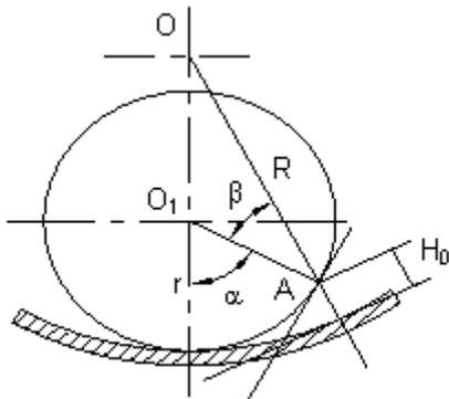
**Fig. 3.** Relationship between the material thickness and die & roller size
