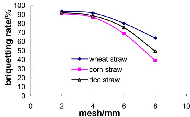
**Fig. 8.** Relationship between granularity and briquetting rate with three kinds of straws
