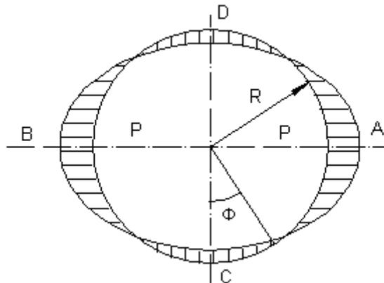
Fig. 5. Chart of bending moment on the ring die
