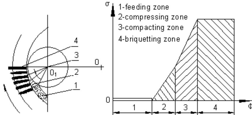
Fig. 2. Compressing force in different region of the raw material
