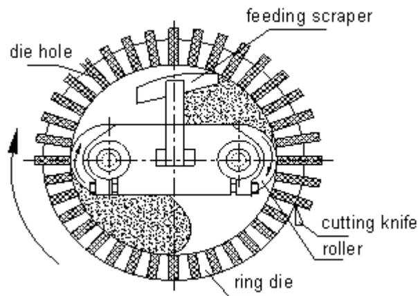
Fig. 1. Theoretical chart of ring die pellet mill
