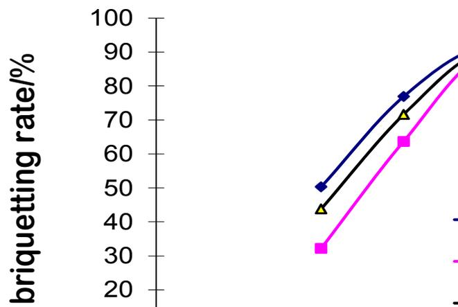
**Fig. 9.** Relationship between moisture ratio and briquetting rate with three kinds of straws
