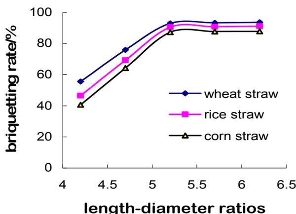
**Fig. 10.** Relationship between length diameter ratio and briquetting rate with three kinds of straws
