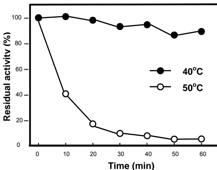
**Fig. 5.** Thermal stability of *KRICT PX2* xylanase. The enzyme was maintained for 1 hour at 40 and 50°C, and residual activity was measured at 10 minute intervals under standard assay conditions.
