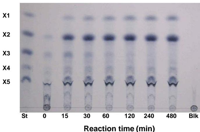
**Fig. 6.** TLC analysis of the products after hydrolysis of birch wood xylan (0.5%) by *KRICT PX2* xylanase (160  $\mu\text{g}/\text{mL}$ ) for each reaction time of 0, 15, 30, 60, 120, 240, and 480 minutes in a 50mM glycine buffer (pH 9.0) at 40°C. St: xylo-oligomer standards, X1: xylose, X2: xylobiose, X3: xylotriose, X4: xylotetrose, X5: xylopentose, respectively. Blk: blank without xylanase
