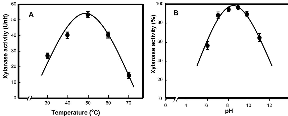
**Fig. 3.** The xylanase activity of *KRICT PX2* at various temperature (A) and pH (B) conditions. The enzyme activity was assayed at 50°C in 50 mM citric buffer (pH 2~6.5), phosphate buffer (pH 7~9), and glycine buffer (pH 9.5~12), and also assayed at different temperature in 50 mM citric buffer (pH 5.5), and glycine buffer (pH 9.5), respectively.
