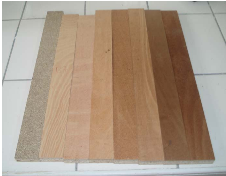
Fig. 1. Laminated and non-laminated bending test samples
