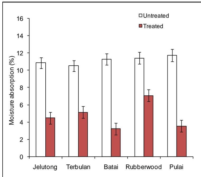
Fig. 3. Moisture absorption of untreated and treated wood samples
