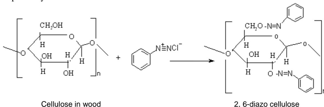
**Fig. 1.** The coupling reaction scheme of benzene diazonium chloride with cellulose unit
