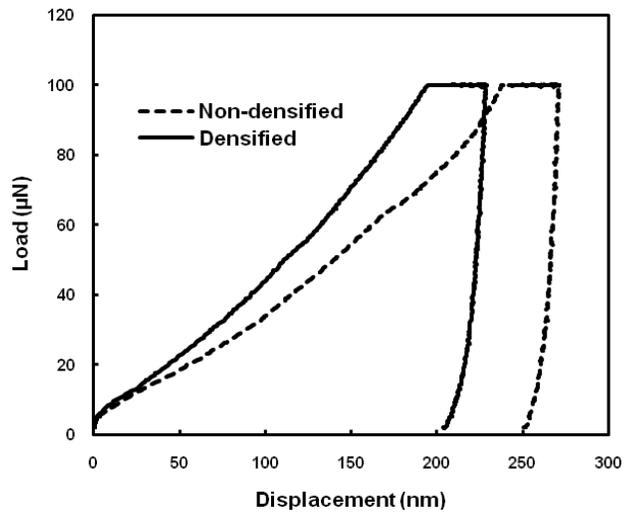
**Fig. 1.** Typical load-displacement curves of nanoindentations in fiber cell walls of trembling aspen non-densified without oil-heat treatment (control) and densified at 200°C with oil-heat treatment at 220°C
