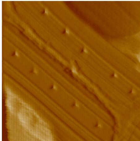
**Fig. 2.** Typical nanoindentations in fiber cell walls of trembling aspen densified at 220°C without oil-heat treatment
