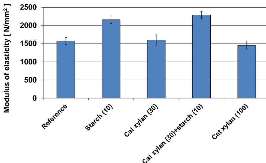
Fig. 14. Dry paper elastic modulus values of the studied samples
