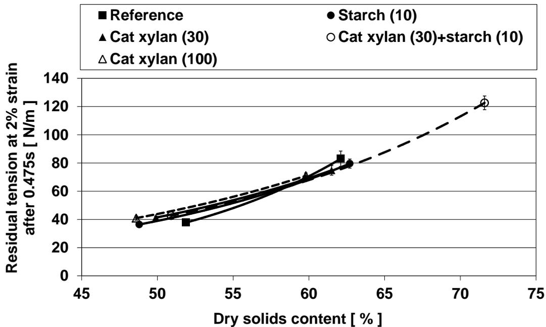
Fig. 11. Wet paper residual tension values with exponential fits
