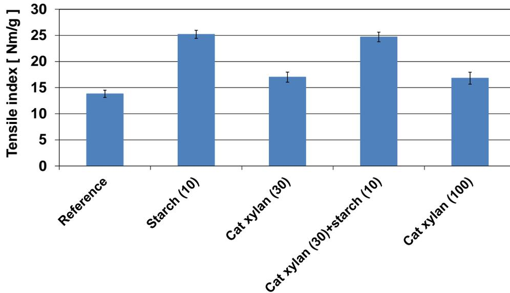
Fig. 12. Dry paper tensile index values of the studied samples
