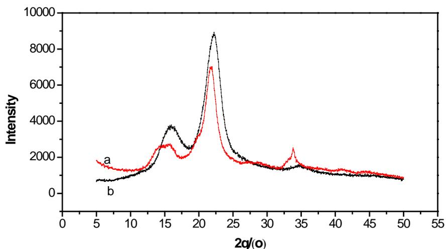
**Fig. 5.** X-ray diffraction image of bamboo nanocrystalline cellulose (a) and cotton nanocrystalline cellulose (b)
