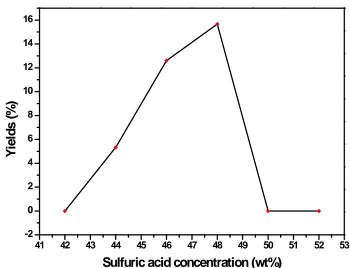
**Fig.1.** Effect of sulfuric acid concentration on yields
