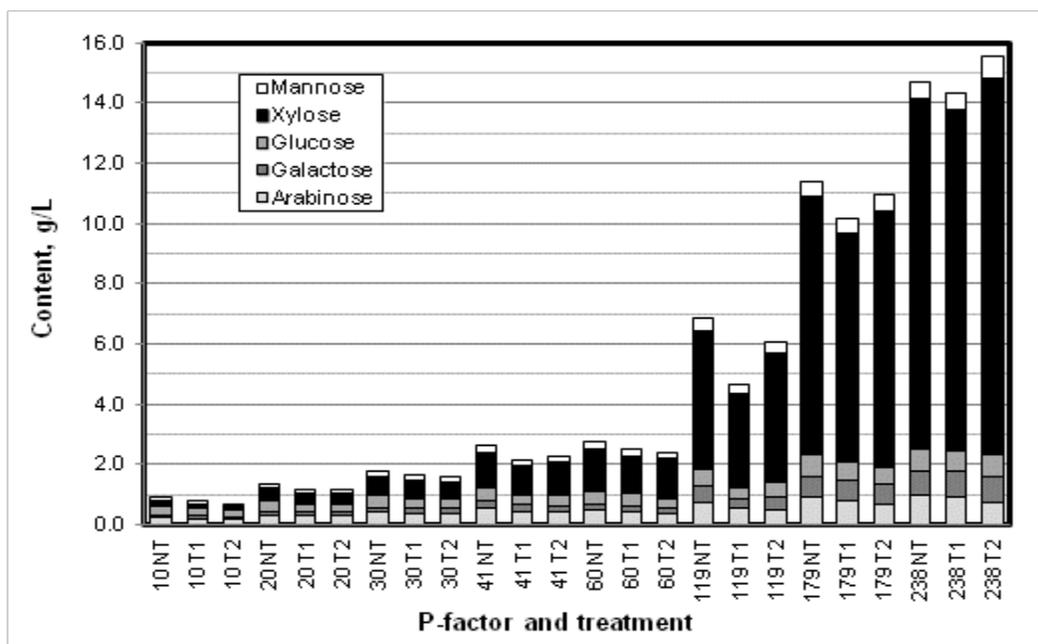
**Fig. 5.** Content of the total carbohydrates in different hydrolysates not treated with XAD-4 (NT), hydrolysates treated with neutral XAD-4 (T1), and hydrolysates treated with basic XAD-4 (T2). The numbers on the horizontal axis labels refer to the P-factor (10–238).
