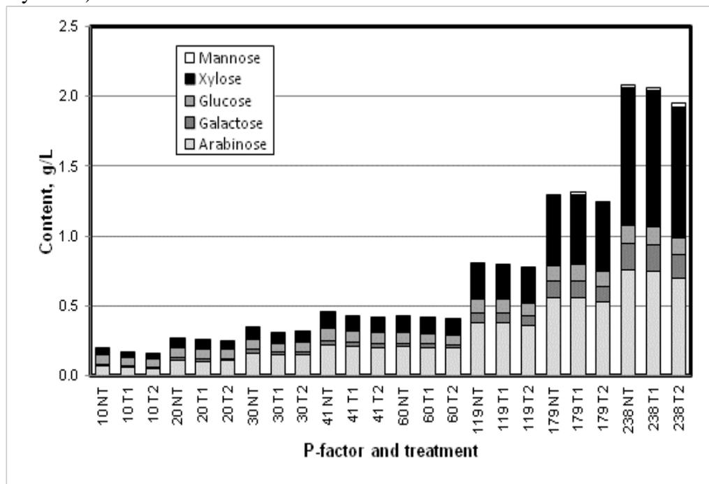
**Fig. 4.** Content of the free monosaccharides in different hydrolysates not treated with XAD-4 (NT), treated with neutral XAD-4 (T1), and treated with basic XAD-4 (T2). The numbers on the horizontal axis labels refer to the P-factor (10–238).
