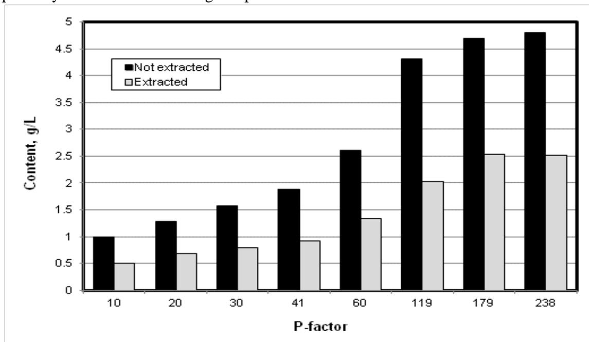
**Fig. 3.** Content of the dissolved lignin in different hydrolysates before and after ethyl acetate extraction
