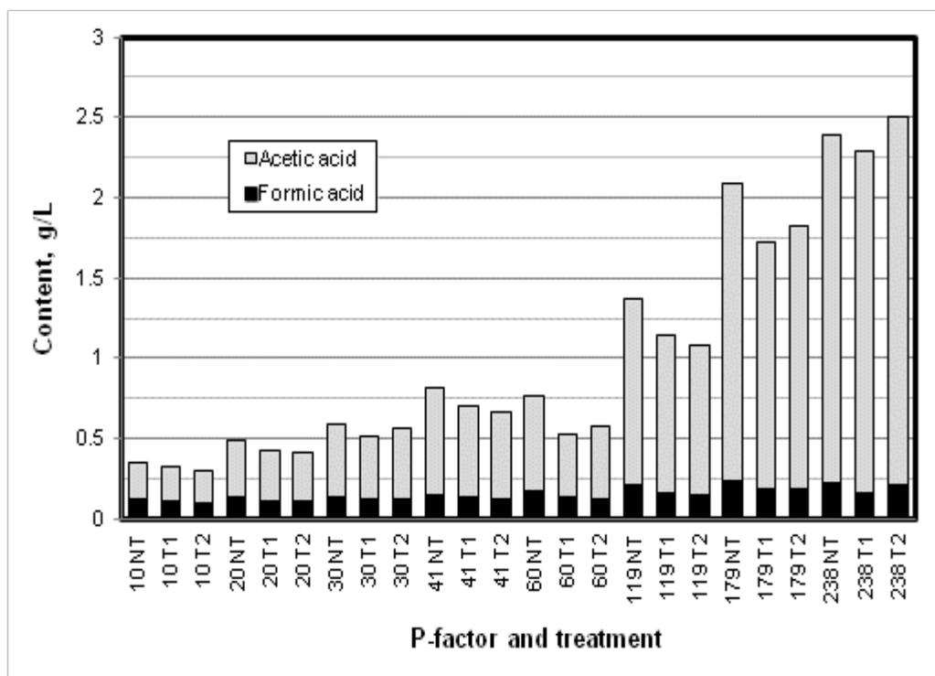
**Fig. 8.** Contents of volatile acids in hydrolysates not treated with XAD-4 (NT), hydrolysates treated with neutral XAD-4 (T1), and hydrolysates treated with basic XAD-4 (T2). The numbers on the horizontal axis labels refer to the P-factor (10–238).
