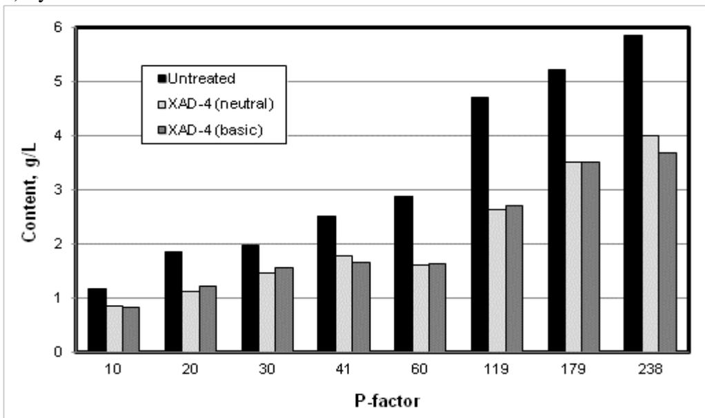
**Fig. 6.** Content of the dissolved lignin in different hydrolysates before and after the XAD-4 treatments
