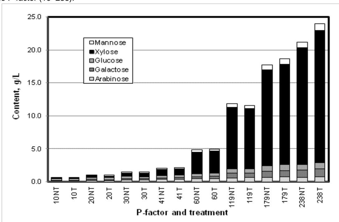
**Fig. 2.** Content of the total carbohydrates in different hydrolysates not treated (NT) and treated (T) with the ethyl acetate extraction. The numbers on the horizontal axis labels refer to the P-factor (10–238).
