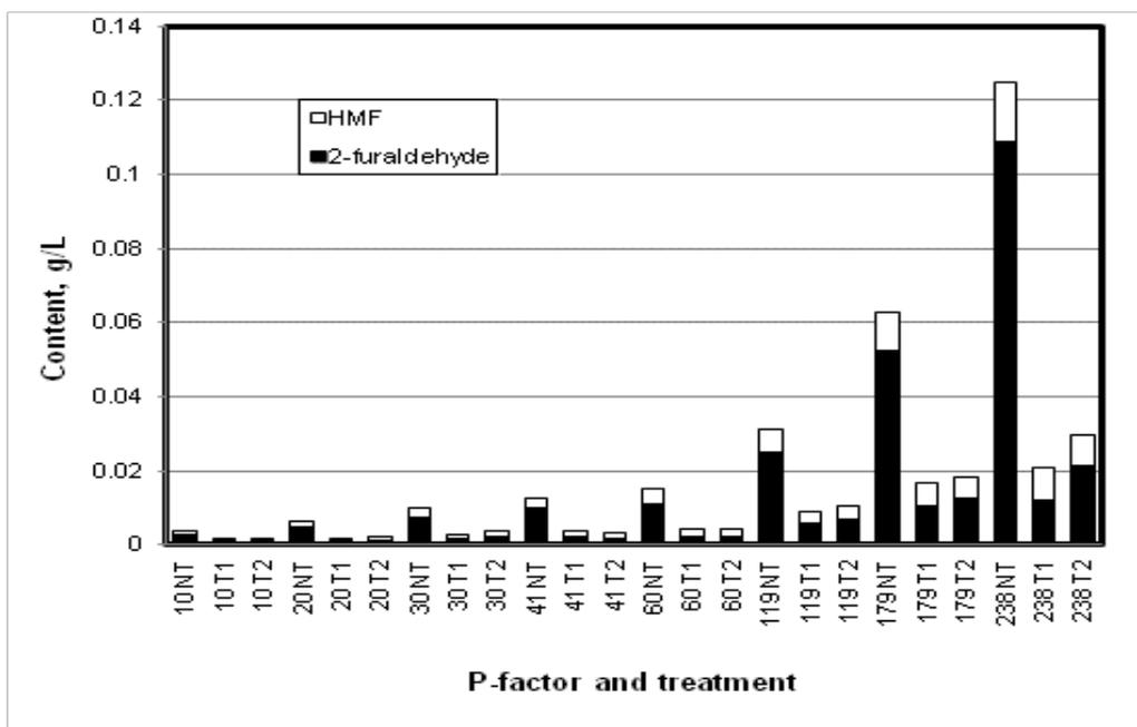
**Fig. 7.** Content of 2-furaldehyde and HMF in different hydrolysates not treated with XAD-4 (NT), hydrolysates treated with neutral XAD-4 (T1), and hydrolysates treated with basic XAD-4 (T2). The numbers on the horizontal axis labels refer to the P-factor (10–238).
