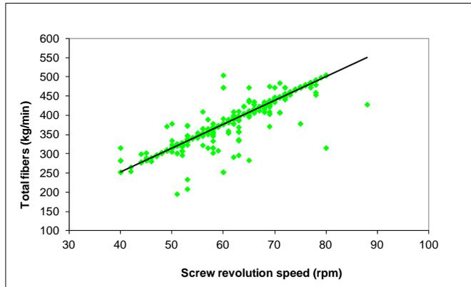
**Fig. 3.** The relationship between the total fibers and the feeding screw revolution speed
