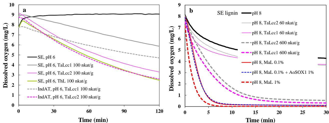
**Fig. 1. a)** Oxygen consumption of SE lignin and Indulin AT solution (ds. 1%) with and without laccase at pH 6. **b)** Oxygen consumption of SE lignin solution (ds. 2.5%) with and without laccase (and AoSOX1) at pH 8. 0.1% MaL dose equals to 31 nkat/g, and 1% MaL dose equals to 310 nkat/g. 1% AoSOX1 dose with respect to sulfur in lignin
