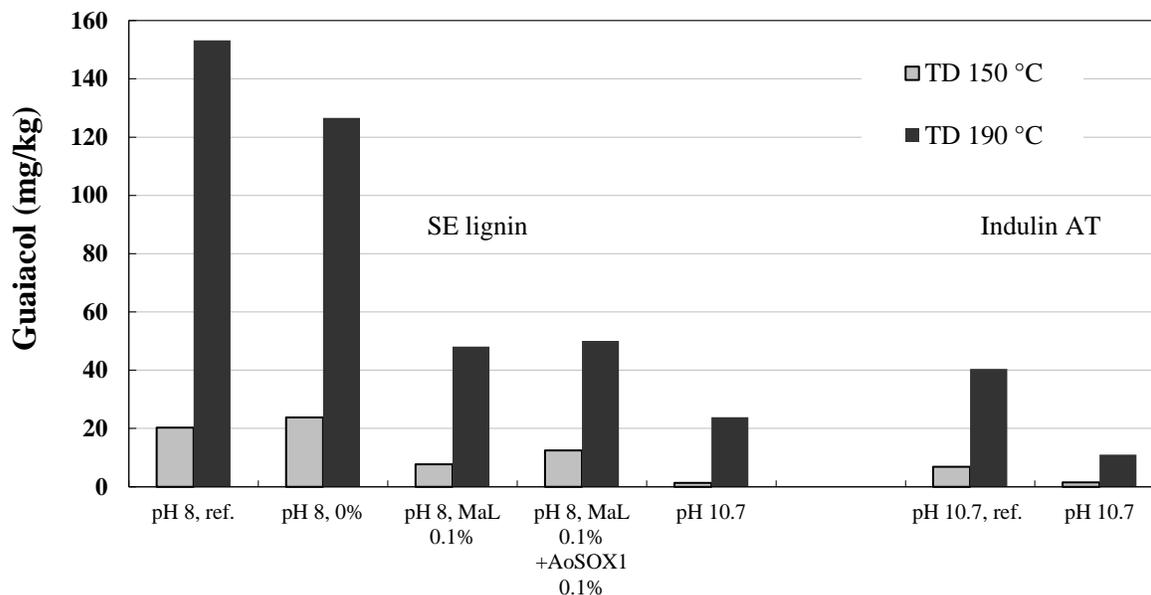
**Fig. 5.** Volatile guaiacol of freeze-dried SE lignin and Indulin AT samples at 150°C and 190°C. Reference samples (ref.) were not O<sub>2</sub> boosted
