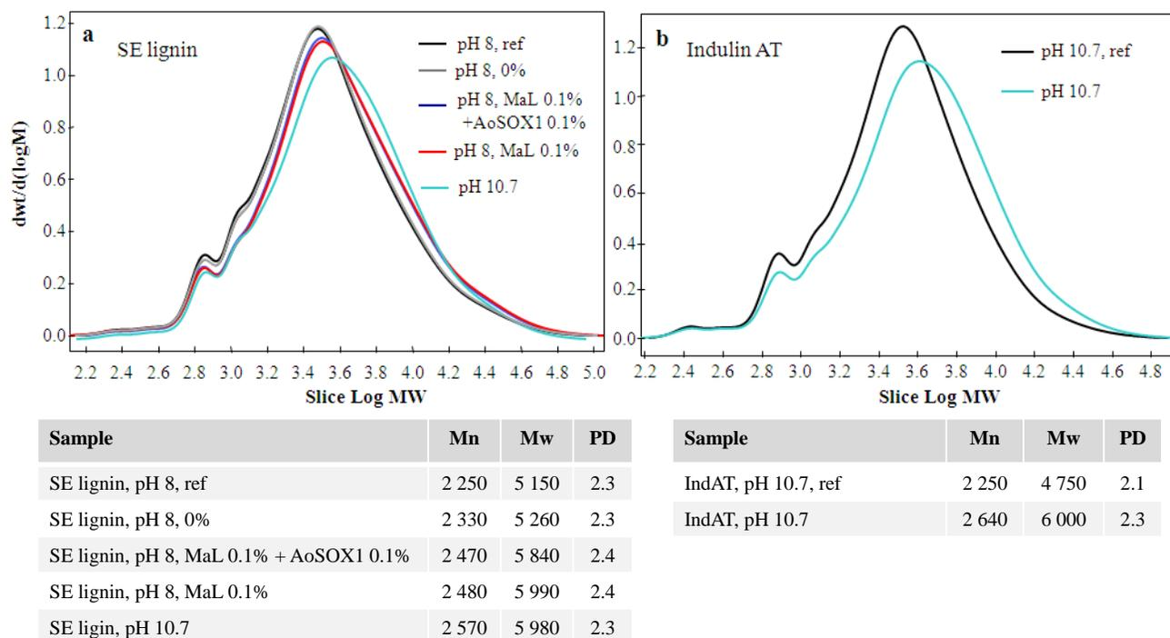
**Fig. 6. a)** Molecular size distributions of freeze-dried SE lignin samples. **b)** Molecular size distributions of freeze-dried Indulin AT samples. Reference samples (ref.) were not O<sub>2</sub> boosted
