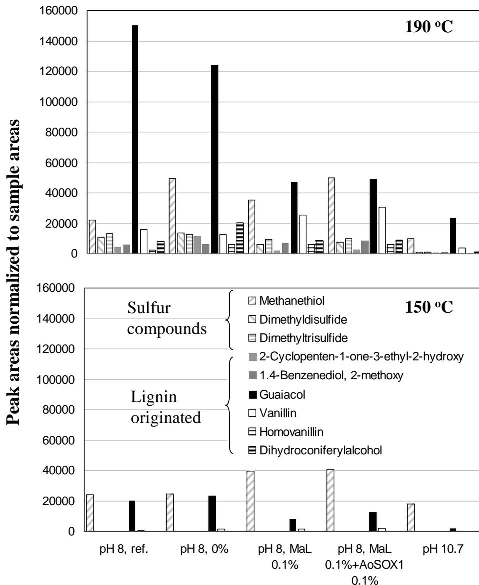
**Fig. 4.** Main volatiles of freeze-dried SE lignin samples at 190°C (upper panel) and 150 °C (lower panel). Reference sample (ref.) was not O<sub>2</sub> boosted
