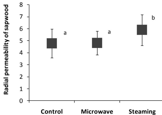
**Fig. 2.** Radial permeability of the sapwood for different treatments of control, microwave-pretreated, and steam-pretreated ( $\times 10^{-16} \text{ m}^3 \text{ m}^{-1}$ )
