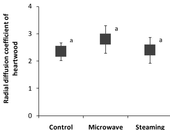
**Fig. 6.** Radial diffusion coefficient in the heartwood treated specimens toward the control ones ( $\times 10^{-7}$ )
