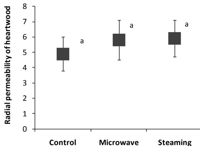
**Fig. 3.** Radial permeability of the heartwood for different treatments of control, microwave-pretreated, and steam-pretreated ( $\times 10^{-16} \text{ m}^3 \text{ m}^{-1}$ )
