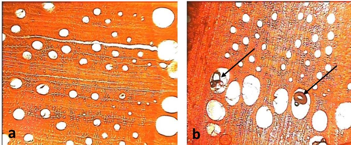
**Fig. 4.** Light microscope feature of sapwood (a) and heartwood (b) of *Q. infectoria* (arrows show the tyloses blocking the way for fluid flow)
