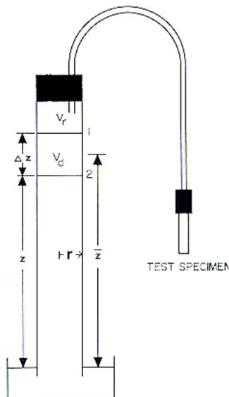
**Fig. 1.** Schematic view of the air permeability measurement apparatus (Taghiyari & Sarvari Samadi 2010) (USPTO No. US 8,079,249, B2; Pub. No. 2010/0281951 A1)
