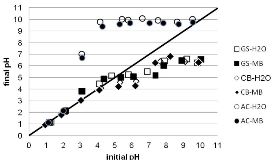
**Fig. 2.** Plot of initial versus final pH solution after contact with activated carbon (AC), grape stalks (GS) and cork bark (CB) in the presence of methylene blue (-MB) and in the absence of MB (-H<sub>2</sub>O). Concentration: 100 mg L<sup>-1</sup>; agitation time: 90 min
