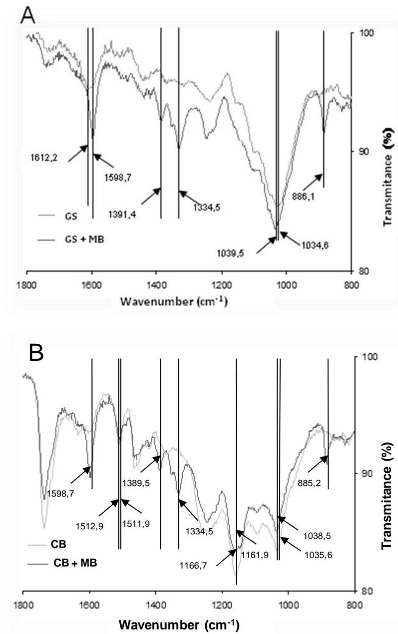
Fig. 5. FTIR spectra of A) grape stalks (GS) and B) cork bark (CB) loaded with methylene blue
