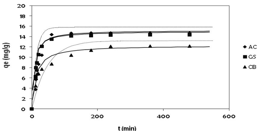
**Fig. 3.** Methylene blue (MB) sorption onto activated carbon (AC), grape stalks (GS), and cork bark (CB) as a function of time. Initial metal concentration:  $100 \text{ mg L}^{-1}$ ; initial pH: 6.5. Symbols are the experimental data, solid lines represent predicted data by the pseudo-first model, and dashed lines represent predicted data by the pseudo-second model.
