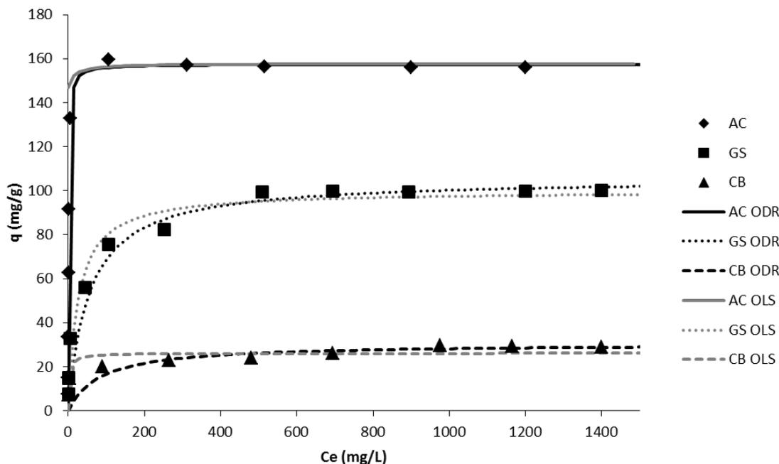
**Fig. 4.** Sorption isotherms of methylene blue (MB) using activated carbon (AC), grape stalks (GS), and cork bark (CB). Solid lines represent predicted data by the Langmuir model, and the symbols are the experimental data. Initial pH = 6.5; contact time (AC) = 240 min; Contact time (AC and GS) = 480 min; T = 20±2°C.
