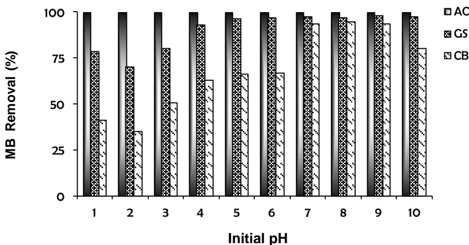
**Fig. 1.** Removal percentage of methylene blue (MB) as a function of solution initial pH by activated carbon (AC), grape stalks (GS), and cork bark (CB). Concentration:  $100 \text{ mg L}^{-1}$ ; agitation time: 90 min
