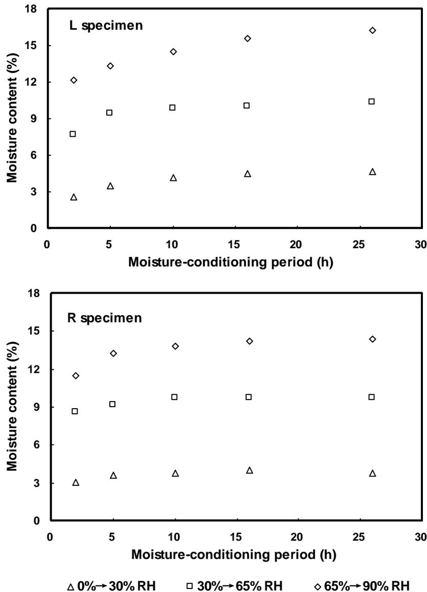
**Fig. 3.** Changes in the moisture content of L and R specimen during the successive adsorption processes
