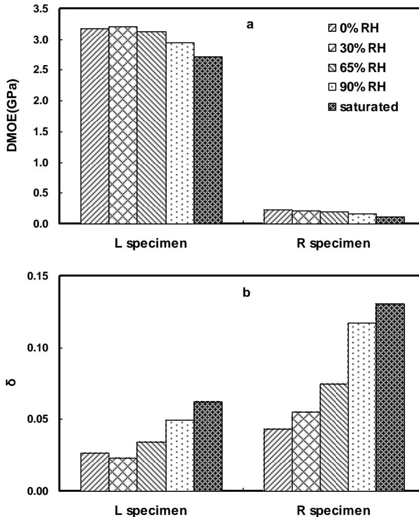
**Fig. 2.** Changes in the DMOE (a) and  $\delta$  (b) of L and R specimens at constant moisture content obtained at various relative humidity levels
