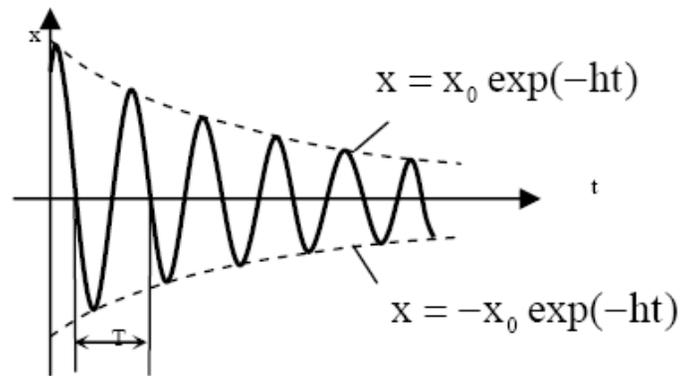
Fig. 1. A typical specimen free vibration response
