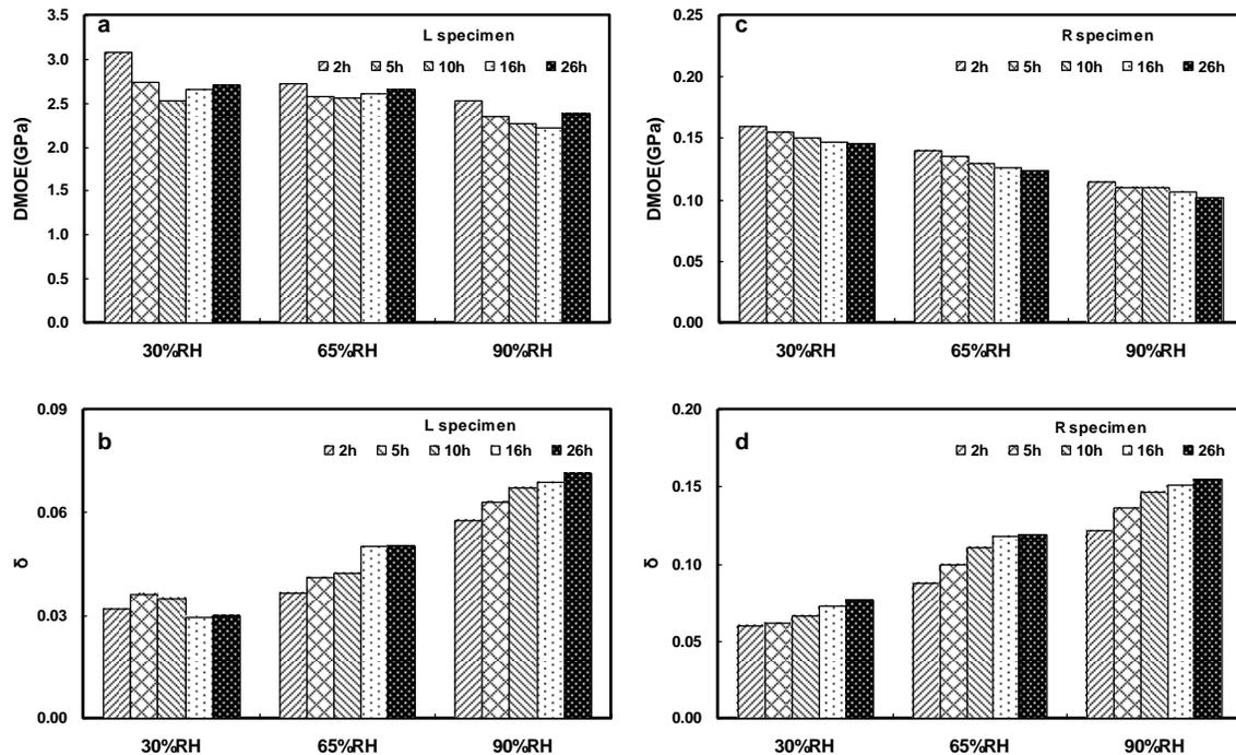
**Fig. 4.** Changes in the DMOE and  $\delta$  of L specimen (a, b) and R specimen (c, d) during the successive adsorption processes
