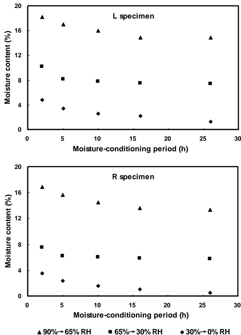
**Fig. 5.** Changes in the moisture content of L and R specimen during the successive desorption processes
