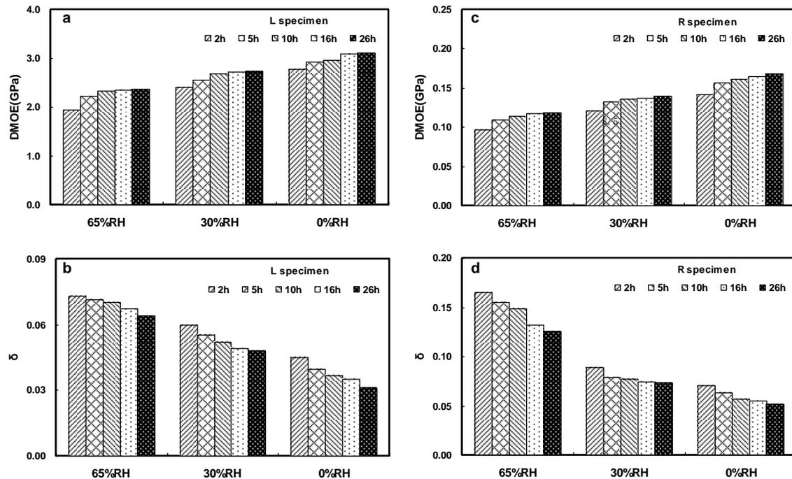
**Fig. 6.** Changes in the DMOE and  $\delta$  of L specimen (a, b) and R specimen (c, d) during the successive desorption processes
