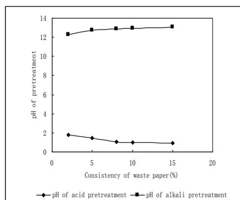
**Fig. 4.** pH of pretreatment vs. varied concentration of pretreatment (Pretreatment time 60 min, waste paper consistency 10% and pretreatment temperature 80 °C)
