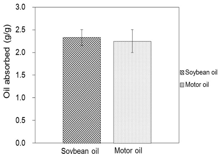
**Fig. 2.** Oil absorption ability of *M. floridulus* stems
