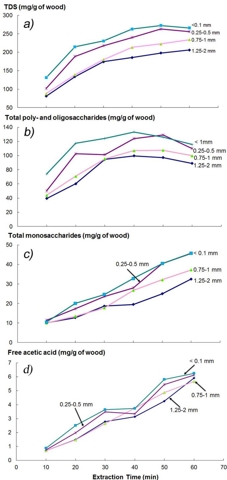
**Fig. 2.** Hot-water extraction yields from wood fractions of different particle size at 170°C: a) total dissolved solids, b) total amounts of poly- and oligosaccharides (calculated as anhydro-sugars based on original dry wood), c) monosaccharides, d) acetic acid released during the extraction
