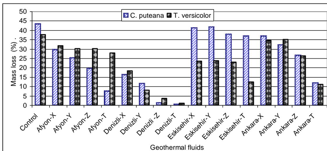
**Fig. 3.** Antifungal effects of GFs prepared at different concentrations against *C. puteana* and *T. versicolor* on wood blocks
