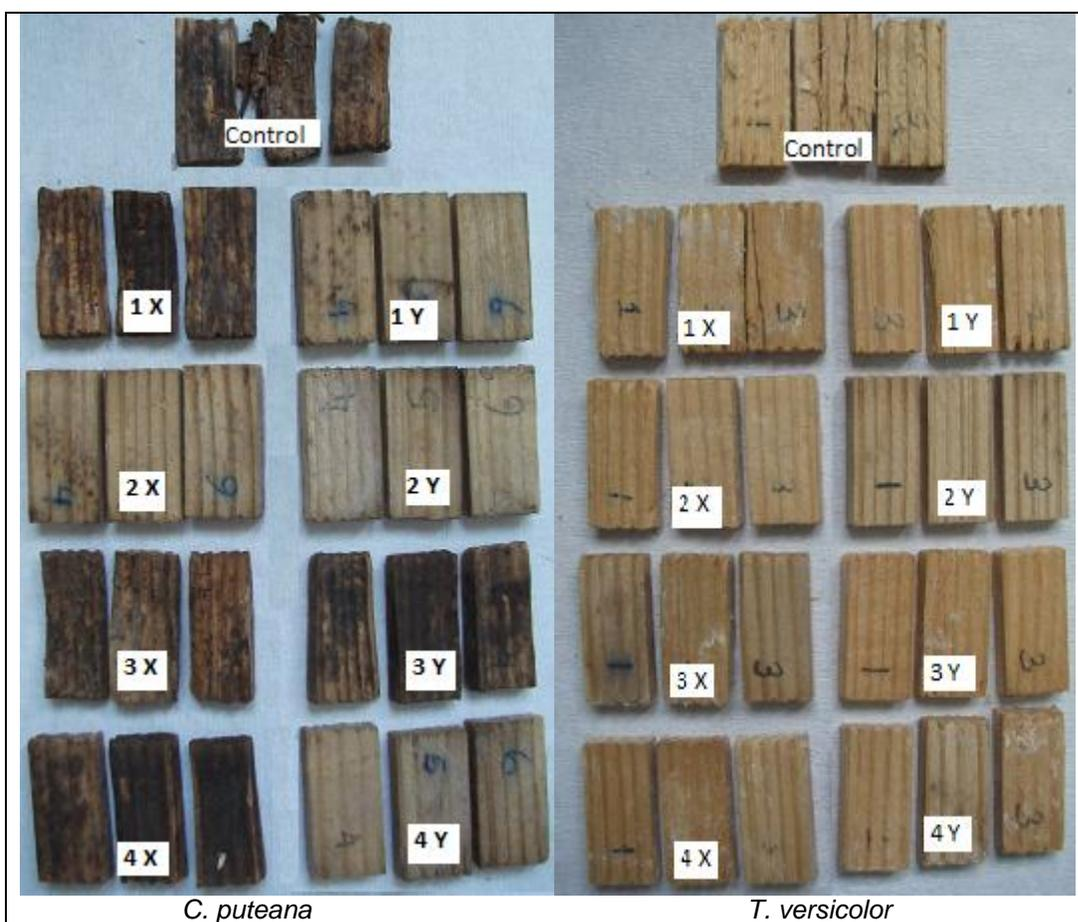
**Fig. 4.** Effects of brown-rot (*C. puteana*) and white-rot (*T. versicolor*) on Scots pine treated with GFs at different concentrations (1: Afyon, 2: Denizli, 3: Eskisehir, 4: Ankara; X: non-concentrated and Y: 75% show the GF evaporation levels)
