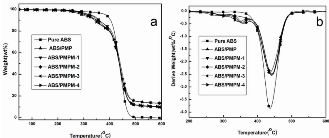
**Fig. 5.** TG (a) and DTG (b) curves of ABS blends in N<sub>2</sub>**Table 3.** Results of TG and DTG Analysis for ABS, ABS/PMP, and ABS/PMPM Blends in N<sub>2</sub> at a Heating Rate of 20 °C /min
