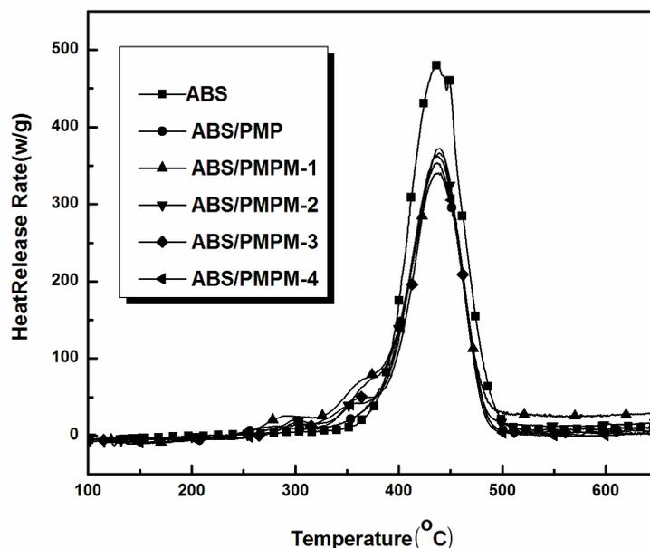
Fig. 6. HRR curves of ABS, ABS/PMP, and ABS/PMPM blends at 1 K/s heating rate
