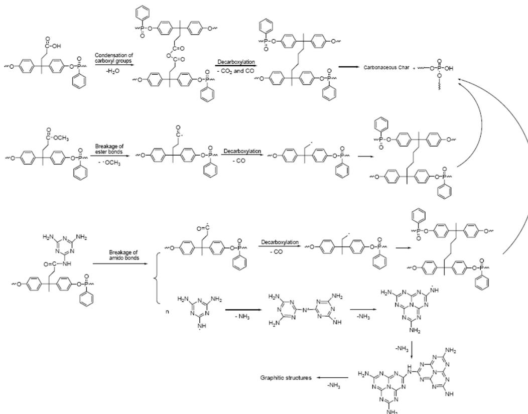
**Fig. 4.** The decomposition mechanisms of PDP, PMP, and PMPM
