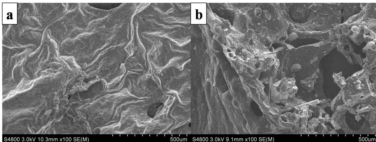
**Fig. 7.** SEM images of the outer surface of the char ( $\times 500$ ): (a) ABS/PMPM-1; (b) ABS/PMPM-4
