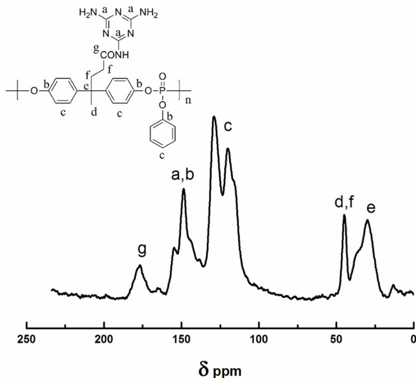
Fig. 1. Solid-state  $^{13}\text{C}$ -NMR spectrum of PMPM-1
