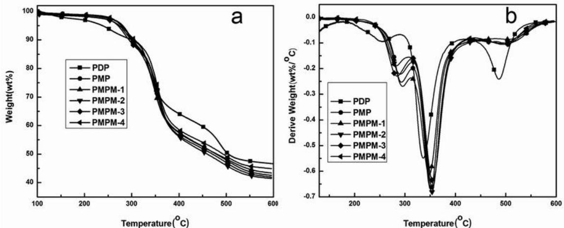
Fig. 3. TG(a) and DTG(b) curves of PDP, PMP, and PMPM flame retardants in  $N_2$
