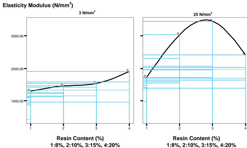
Fig. 2. Elasticity modulus obtained from the bending test
