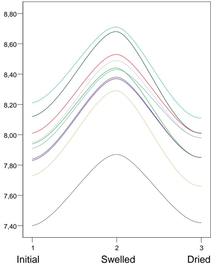
**Fig. 4.** Evolution of the thickness for each sample tested with 20% resin and 25 N/mm<sup>2</sup> pressure
