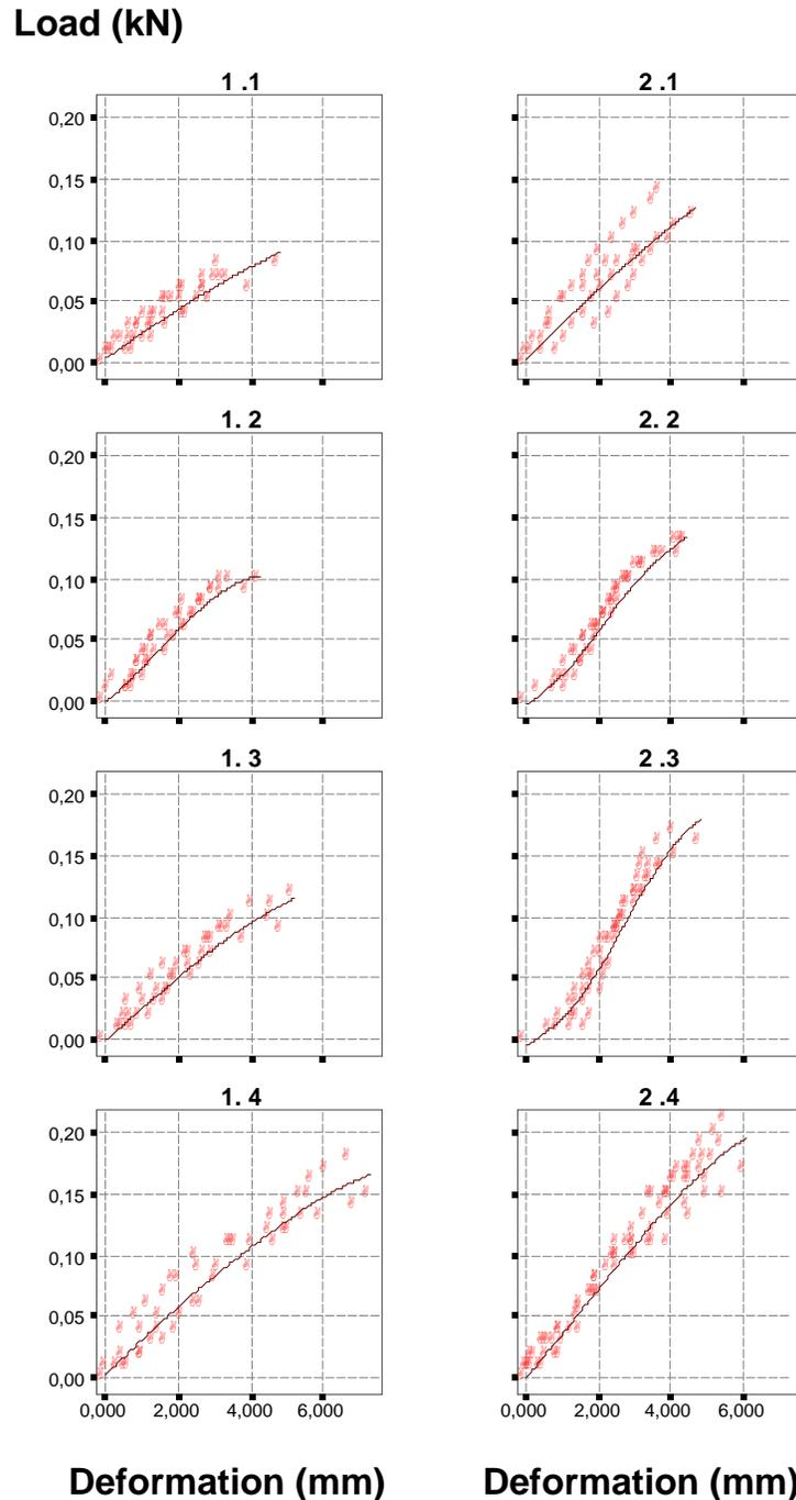
**Fig. 1.** Bending test results for boards developed with different resin contents and pressures applied during manufacturing process
