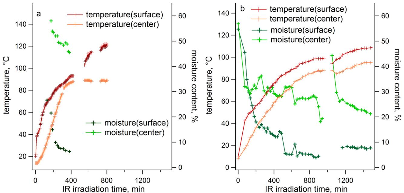
**Fig. 3.** The moisture and temperature profiles of green timbers measured in the surface and the core as a function of IR exposition time. Maximum emitter temperature: **(a)** 165 °C; **(b)** 140 °C
