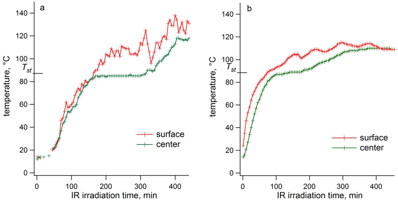
**Fig. 2.** Temperature profiles of green samples of 45-60% initial moisture content as a function of drying time during continuous IR heating exposure. Maximum emitter temperature: **(a)** 165 °C; **(b)** 140 °C
