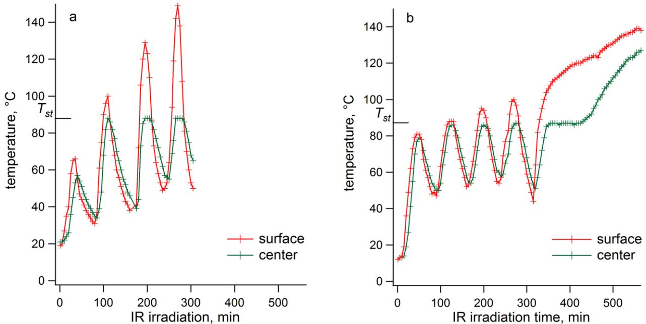
**Fig. 1.** Temperature profiles of green samples of 45 to 60% initial moisture content as a function of drying time during intermittent IR heat exposure. **(a)** Four heating cycles (maximum emitter temperature (165 °C) reached in one step). **(b)** Four heating cycles followed by an approx. 250 min. continuous heating interval (maximum emitter temperature (165 °C) reached through gradual increase)
