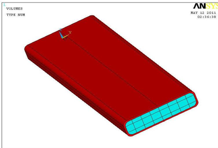
**Fig. 1.** Geometric model for coextruded wood plastic composites
