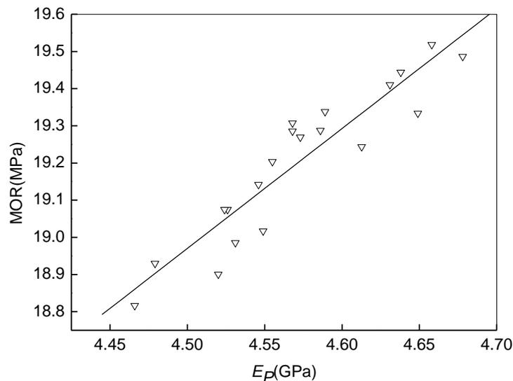
**Fig. 2.** Regression curve between  $E_p$  and MOR of wood-plastic planks of Group 1
