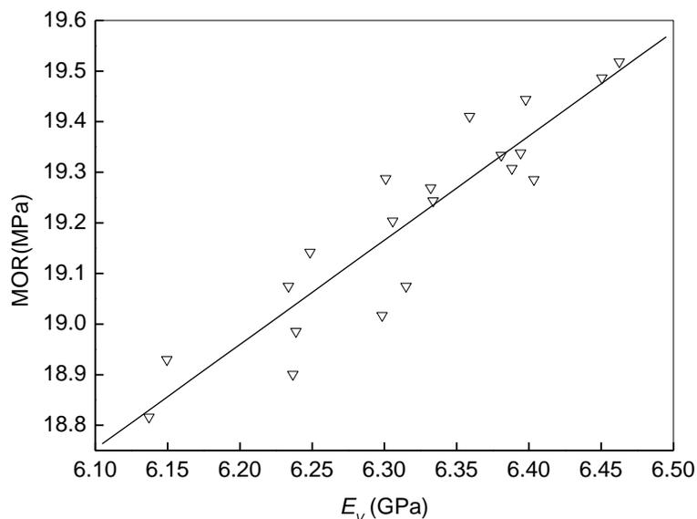
**Fig. 1.** Regression curve between  $E_V$  and MOR of wood-plastic planks of Group 1
