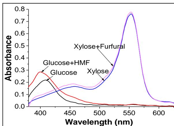
**Fig. 6.** Disturbance from HMF and furfural on sugar analysis. Note: The concentrations of glucose and xylose are both 1.35 mmol/L; the concentrations of furfural and HMF added are both 0.48 mmol/L.
