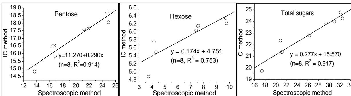
**Fig. 7.** Comparison of the sugar results by both spectrophotometry and IC method
