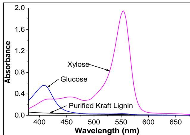
**Fig. 4.** Influence of lignin on sugar analysis. Note: the concentrations of xylose, glucose, and purified kraft lignin are all 0.5 g/L.
