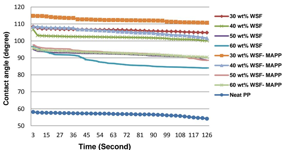
**Fig. 2.** Effects of WSF content and coupling agent (MAPP) on the contact angle of the PP composite (WSF: waste sunflower stalk flour)
