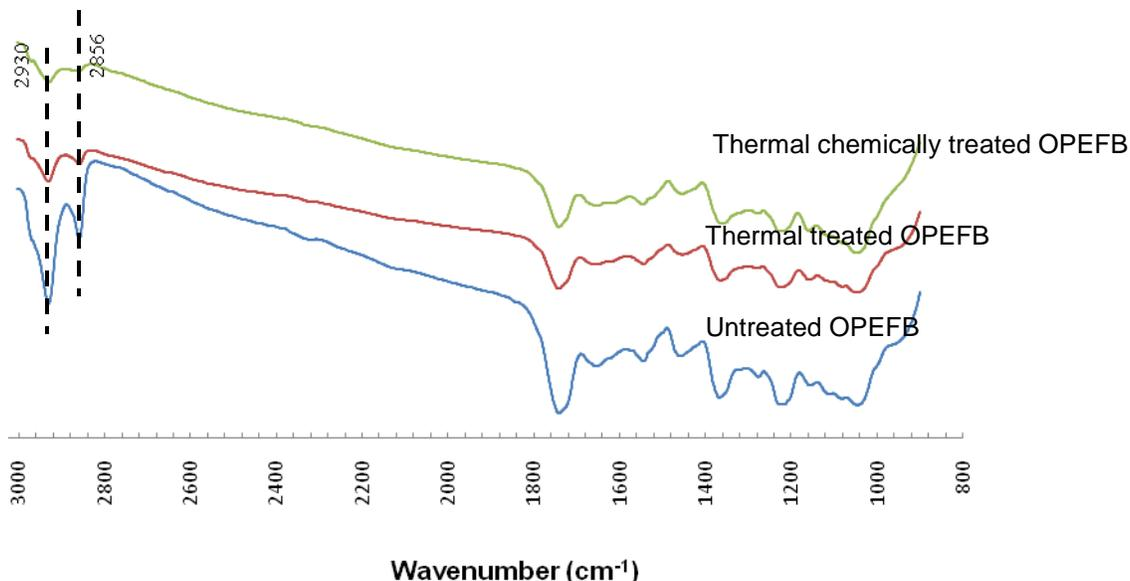
**Fig. 3.** FTIR spectra of treated and untreated OPEFB
