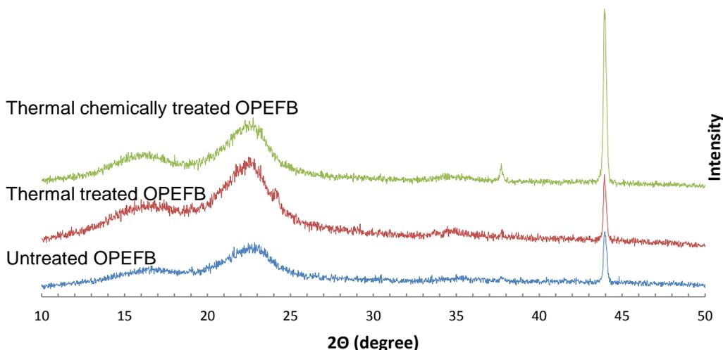
**Fig. 2.** XRD analysis of untreated and treated OPEFB
