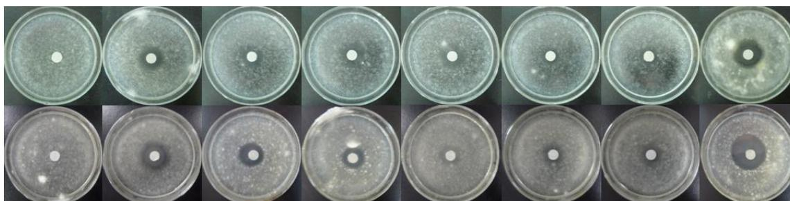
**Fig. 3** Inhibition of the samples to the fungi; From left to right: control, 4a, 4b, 8a, 8b, 8c, 8d and 1227. From top to bottom: *Trametes versicolor* and *Gloeophyllum trabeum*.
