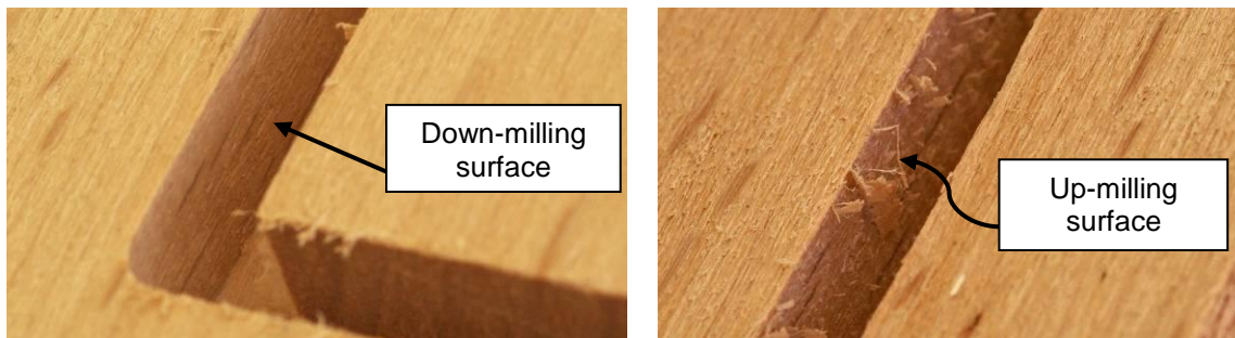
Fig. 4. Comparison of down-milling versus up-milling on the same channel on beech EGP
