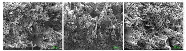
Fig. 5. Fracture behavior of D. barbatus (outer part) depending on modification temperature
