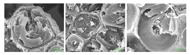
Fig. 6. Fracture behavior of fibers of D. barbatus depending on modification temperature
