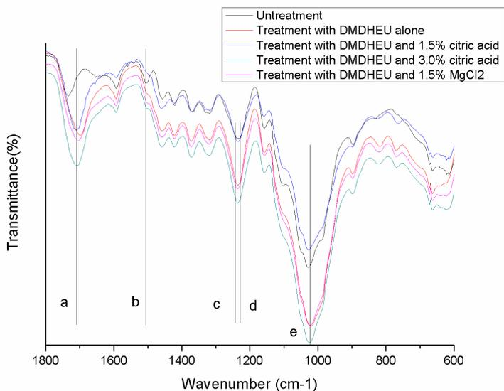
**Fig. 5.** FTIR spectra of DMDHEU-treated and untreated wood powder: (a) carbonyl stretching in wood and DMDHEU; (b) aromatic skeletal vibration in lignin; (c) C-O stretching in lignin and hemicellulose; (d) C-O stretching in lignin and acetyl and carbonyl vibration in hemicellulose, as well as C-O vibration at the N-methylol group of DMDHEU; and (e) C-O stretching in alcohol and ether groups of polysaccharides and lignin.
