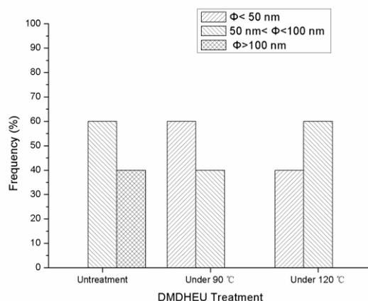
**Fig. 4.** Frequency of pore diameter distribution in wood modified with DMDHEU
