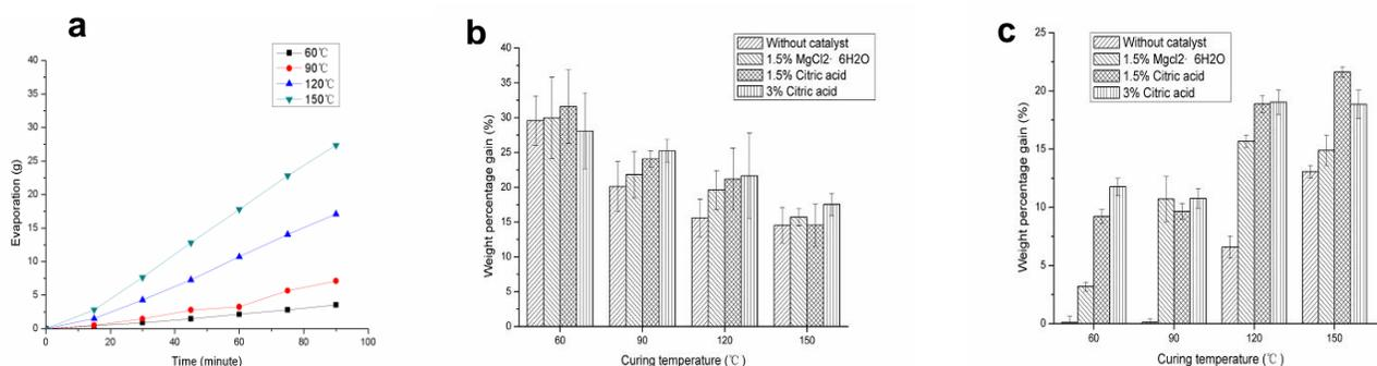
**Fig. 1.** (a) The evaporation of DMDHEU under different temperatures; (b) Weight percentage gain of treated samples; (c) Weight percentage gain of treated samples after leaching. Error bars show standard deviation.
