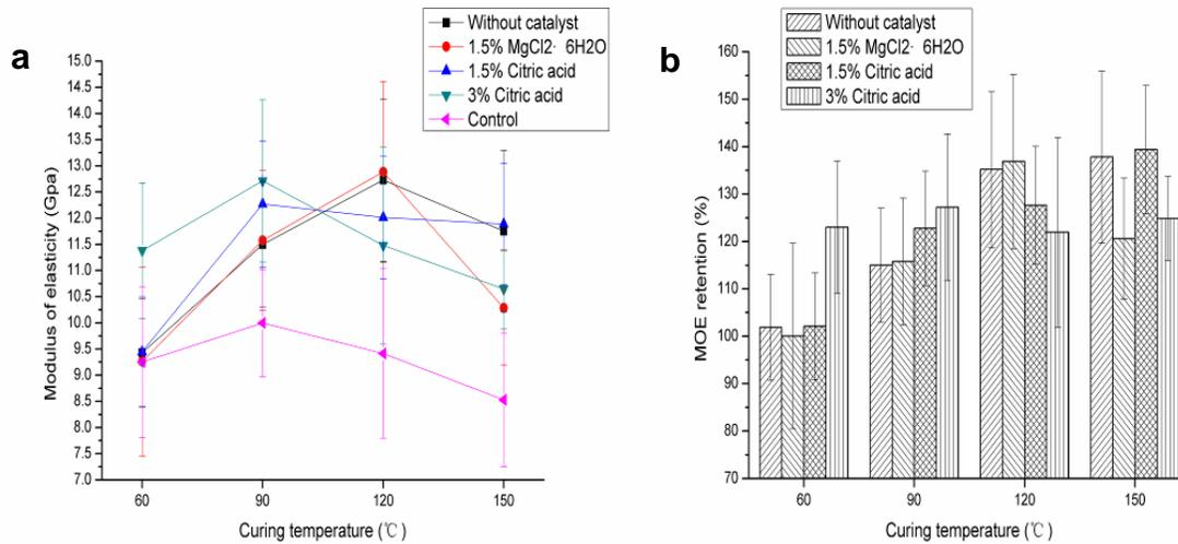
**Fig. 2.** (a) The MOE change of wood treated with DMDHEU and different catalysts under different temperatures; (b) The MOE retention of wood treated with DMDHEU and different catalysts under different temperatures. Error bars show standard deviation.
