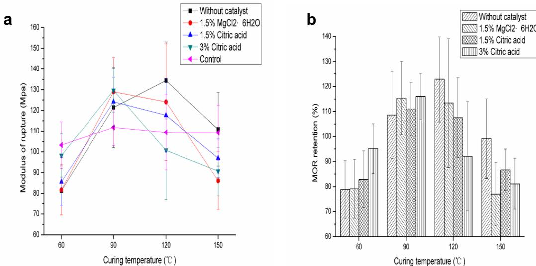
**Fig. 3.** (a) The MOR change of wood treated with DMDHEU and different catalysts under different temperatures; (b) The MOR retention of wood treated with DMDHEU and different catalysts under different temperatures. Error bars show standard deviation.
