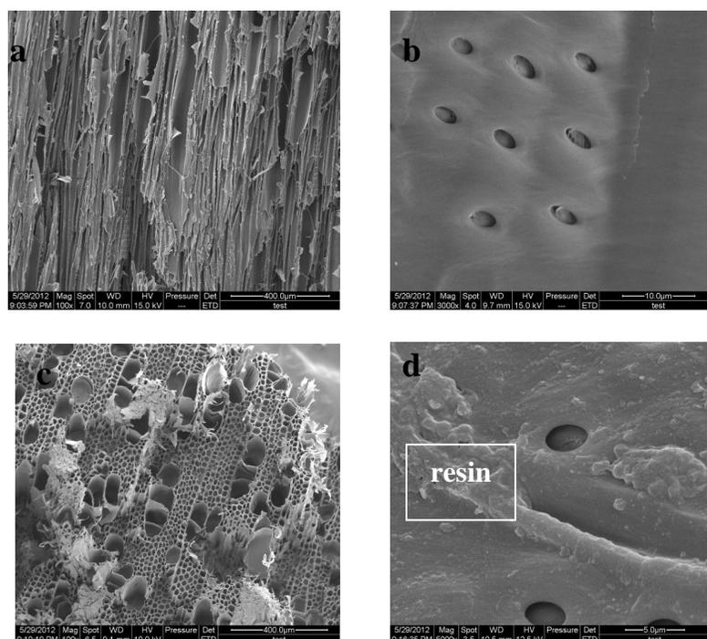
**Fig. 6.** SEM photomicrographs (a) typical failure of treated wood under  $90^{\circ}\text{C}$  (b) nothing on the cell wall of treated wood under  $90^{\circ}\text{C}$  (c) typical failure of treated wood under  $120^{\circ}\text{C}$  (d) resin on the cell wall of treated wood under  $120^{\circ}\text{C}$ .
