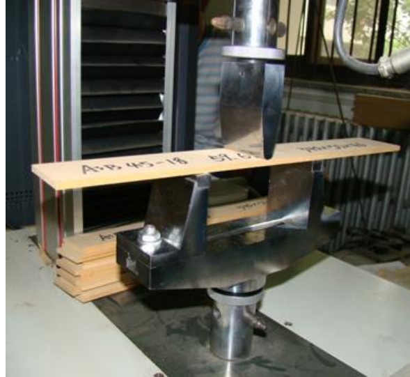
Fig. 5. The mid-point bending test set-up
