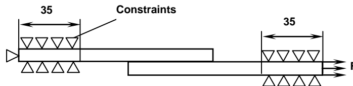
Fig. 3. Loading and constraints of the tensile model of lap joints
