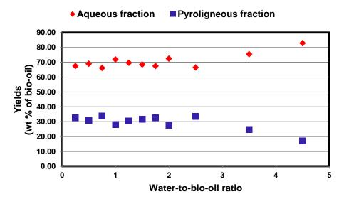
Fig. 1. Effect of the water-to-bio-oil ratio on the yields of aqueous and pyroligneous fractions
