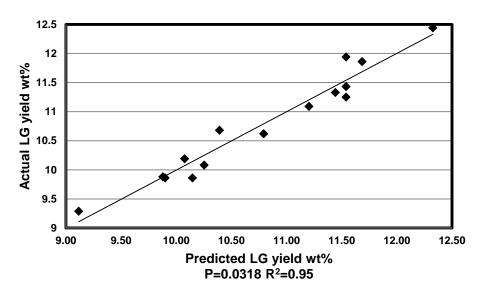
Fig. 4. The relationship between the actual and predicted levoglucosan yield extracted into the aqueous fraction as predicted by regression analysis
