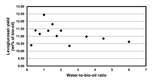
Fig. 3. Effect of the water-to-bio-oil ratio on the yield of levoglucosan
