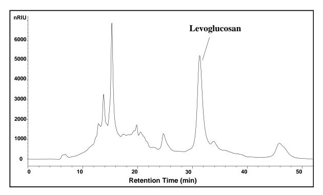
Fig. 2. Liquid chromatogram of a typical bio-oil aqueous fraction sample
