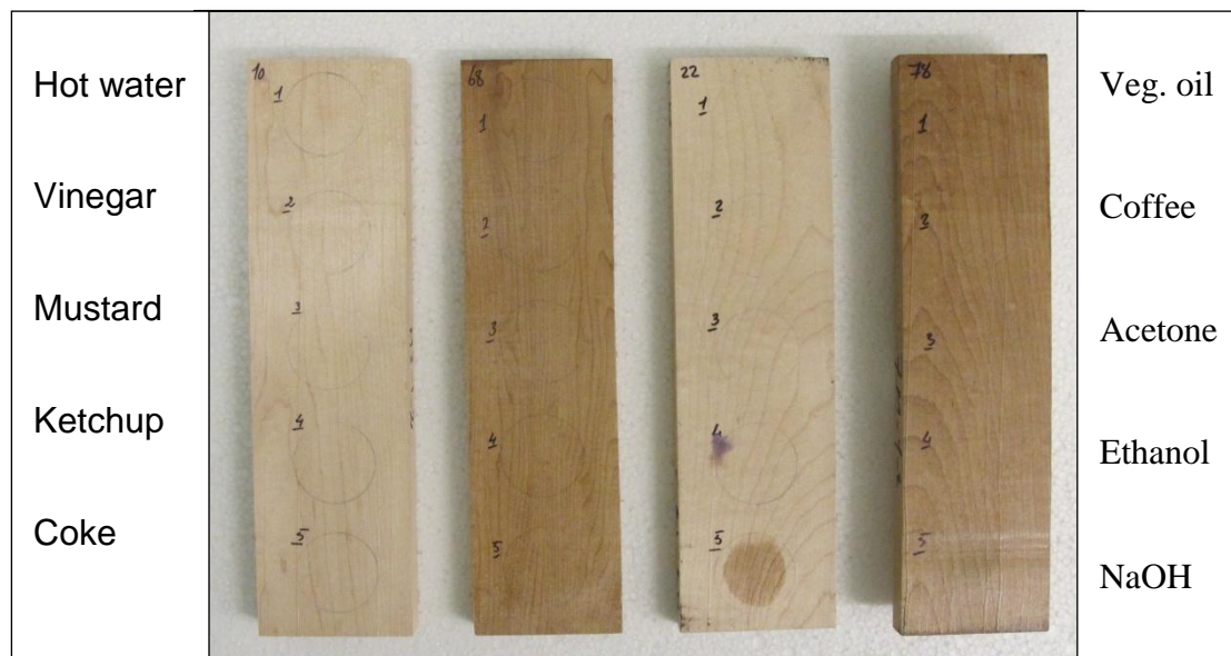
Fig. 4. Stain of mustard on spots number 3 (left–two samples), and stain of alkali solution on spot number 5 (right–two samples).
