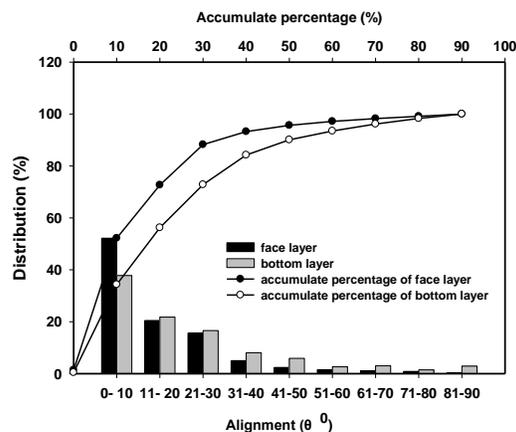
**Fig. 1.** Strand alignment distribution and accumulation percentage of the PF-impregnated OSBs
