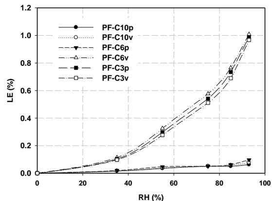
Fig. 5. Linear expansion of the PF-impregnated OSB
