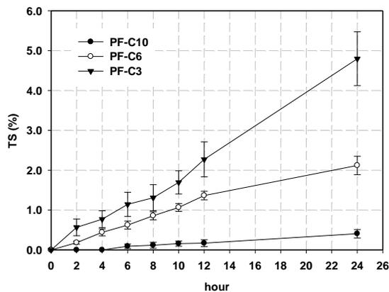
Fig. 4. Thickness swelling of the PF-impregnated OSB
