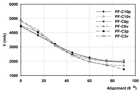
**Fig. 2.** Effects of strand alignment angles ( $\theta^\circ$ ) on the ultrasonic velocity ( $V$ ) of the PF-impregnated OSBs
