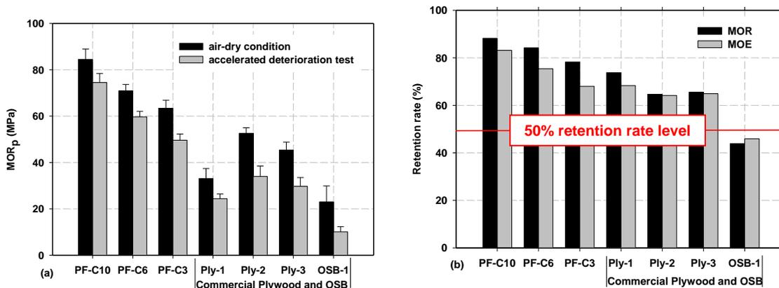
**Fig. 6.** Comparison of the bending properties and strength retention rate of PF-impregnated OSB specimens and commercial structural boards: (a) bending strength, (b) strength retention rate
