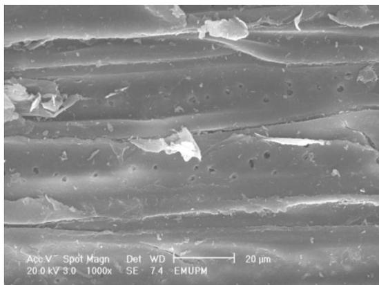
**Fig. 3.** HM pretreated kenaf core V36 under SEM at 1000X magnification
