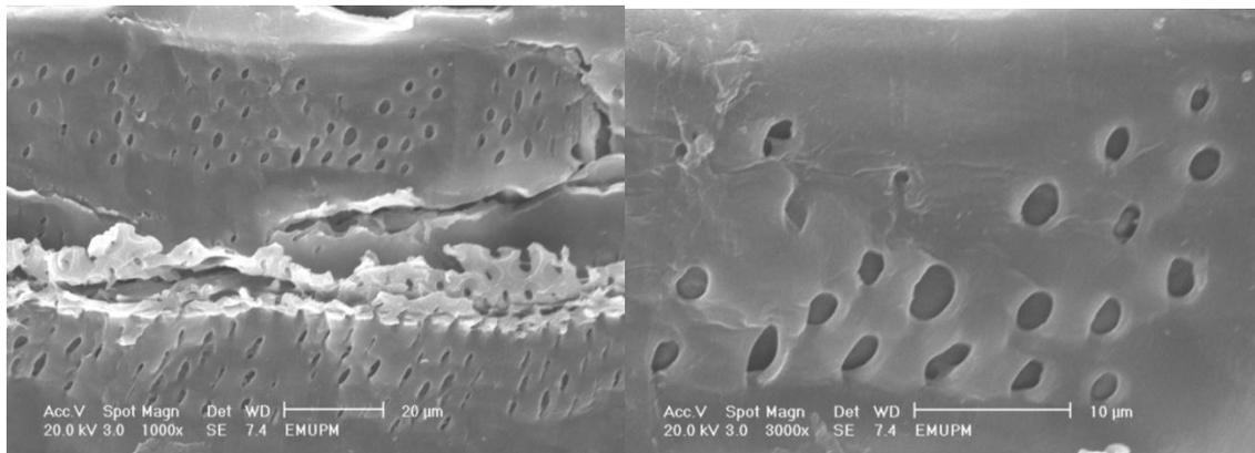
**Fig. 1.** HMCHN-17.5 pretreated kenaf core V36 under SEM at 1000X magnification
