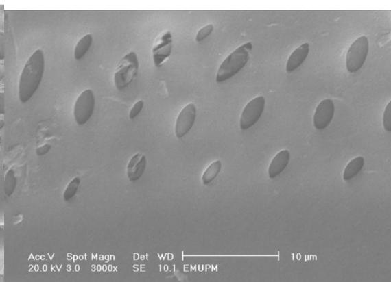
**Fig. 6.** HMTH pretreated kenaf core V36 under SEM at 3000X magnification
