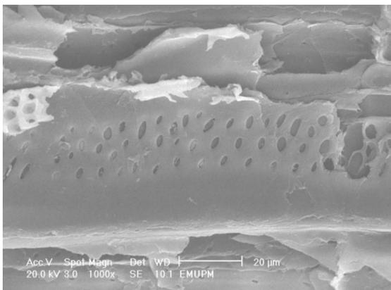
**Fig. 5.** HMTH pretreated kenaf core V36 under SEM at 1000X magnification
