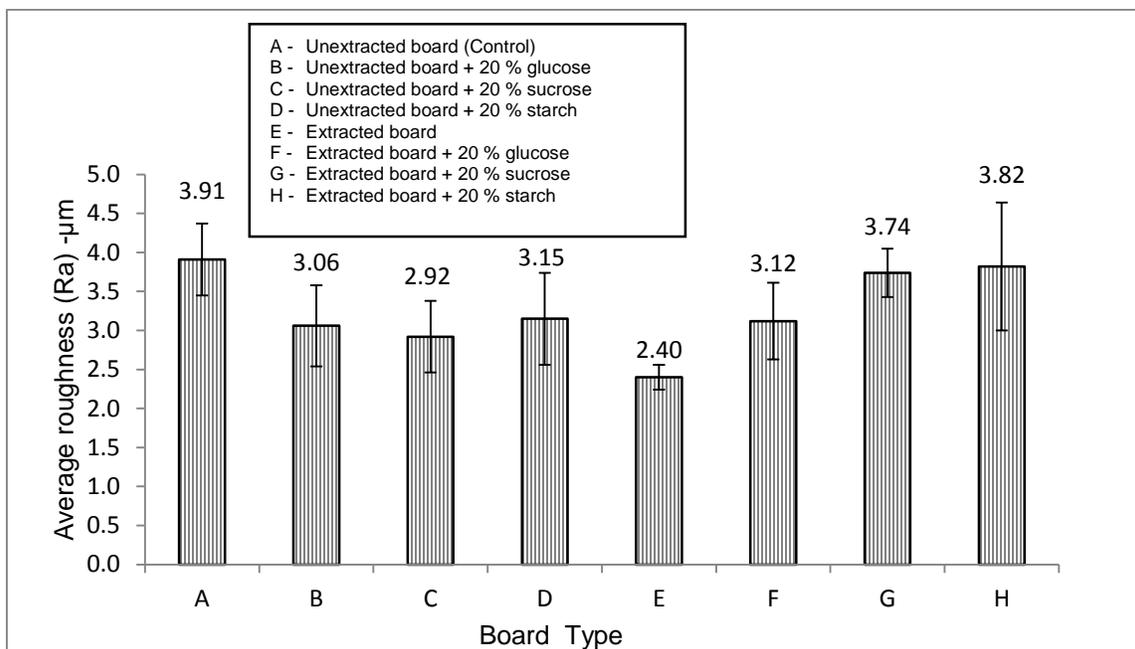
Fig. 4. Average surface roughness ( $R_a$ ) of all type of boards
