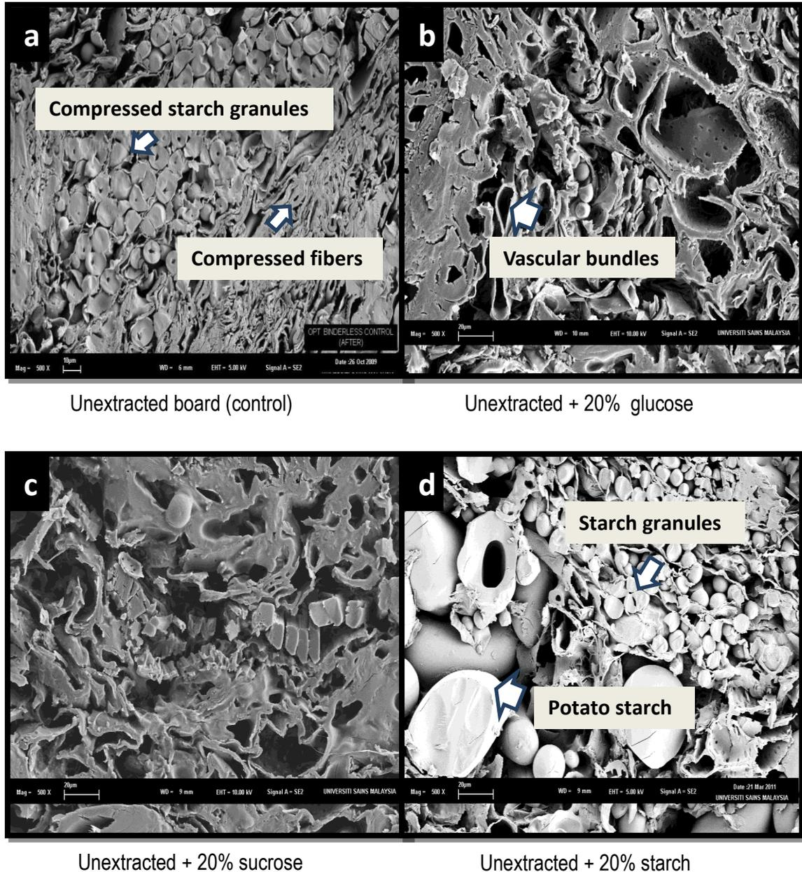
**Fig. 5.** SEM Micrographs of unextracted board and unextracted board with the addition of sugars and starch
