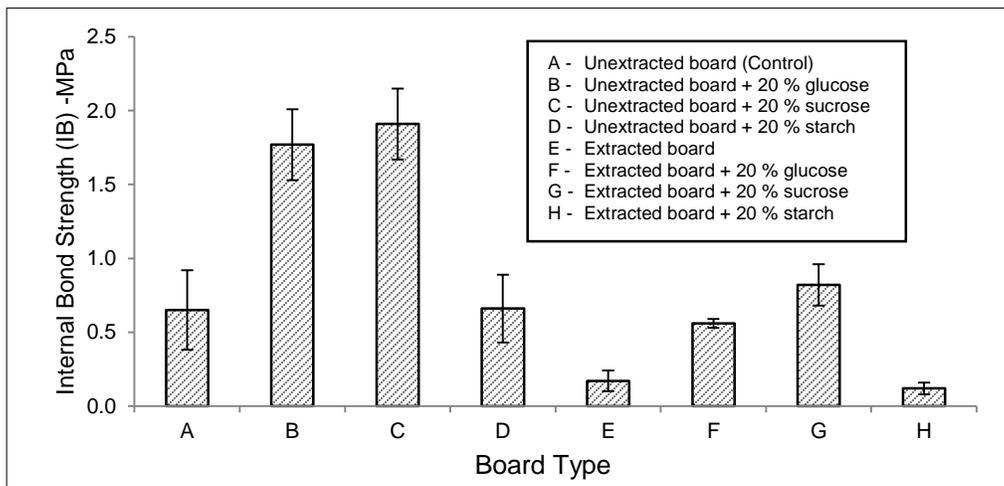
Fig. 2. Internal bond strength of different board types
