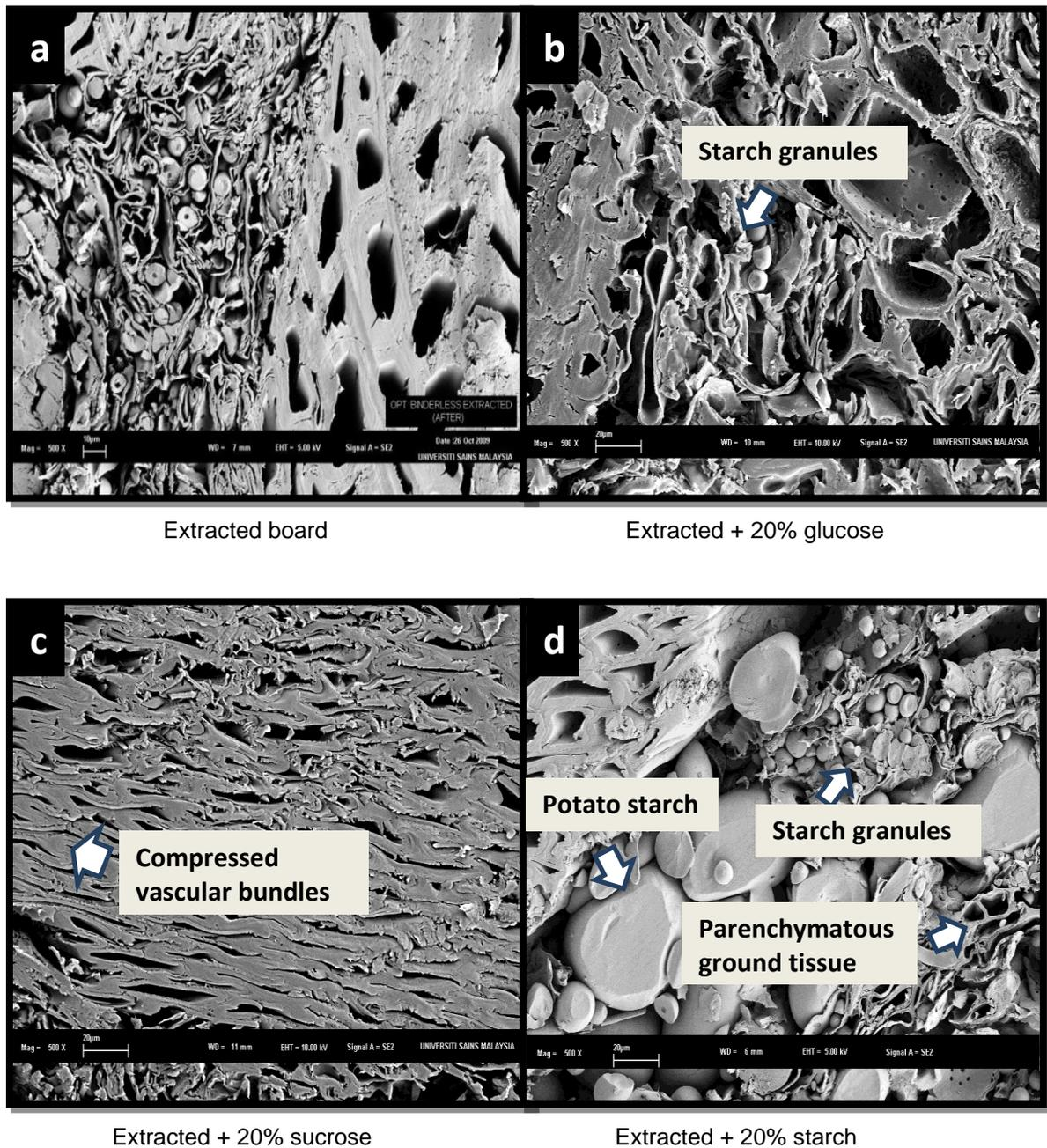
**Fig. 6.** SEM micrographs of extracted board and extracted board with the addition of sugars and starch
