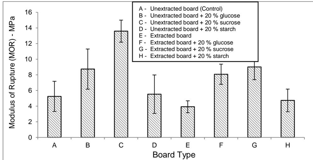
Fig. 1. Modulus of rupture of different panel boards types
