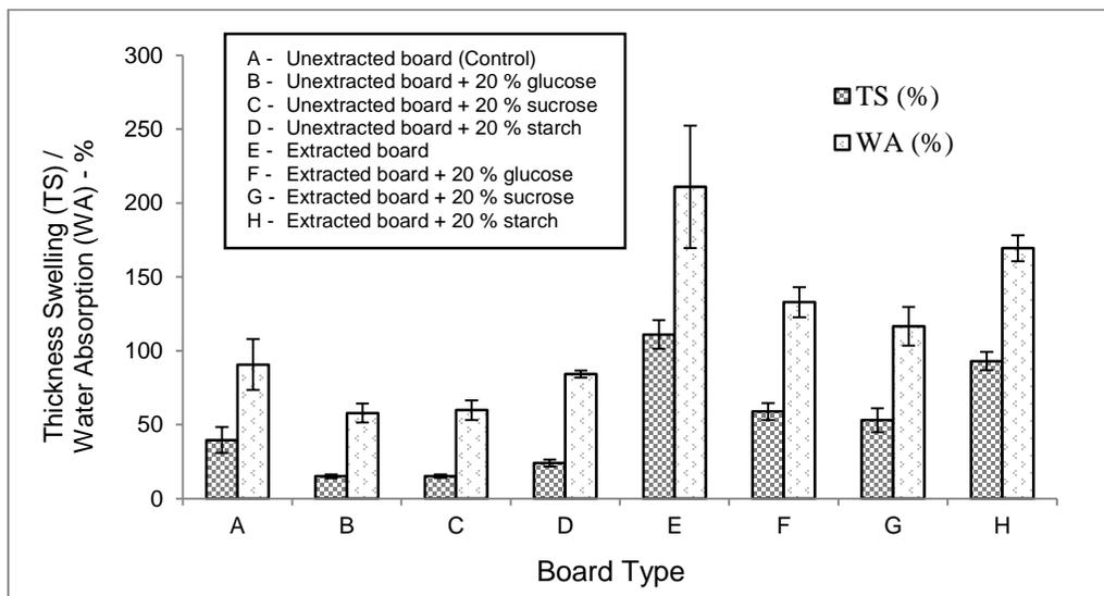
Fig. 3. Thickness swelling and water absorption of different board types
