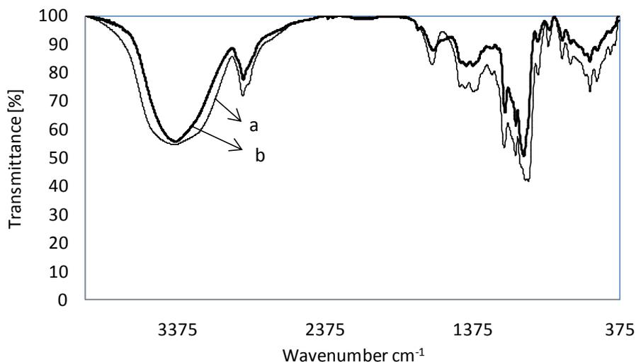
**Fig. 4.** IR spectrums of (a) cassava starch and (b) crosslinking cassava starch
