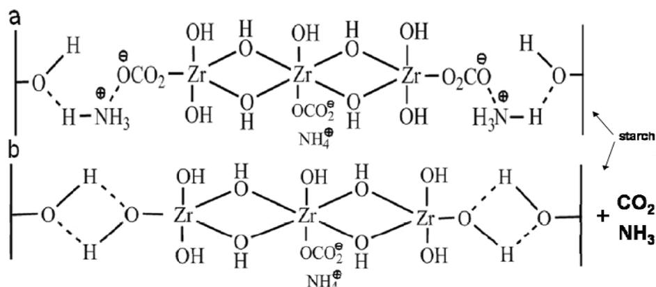
**Fig. 2.** The reaction of AZC with starch. a:  $\text{NH}_4^+$  in AZC reacts with starch *via* hydrogen bonding, linking to basic zirconium carbonate ions *via* ionic attractions; b:  $\text{NH}_3$  and  $\text{CO}_2$  are released during drying, and form new hydrogen bonds between starch and AZC.
