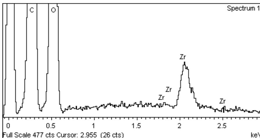
**Fig. 6.** The Energy Diffraction Spectrum of crosslinking cassava starch
