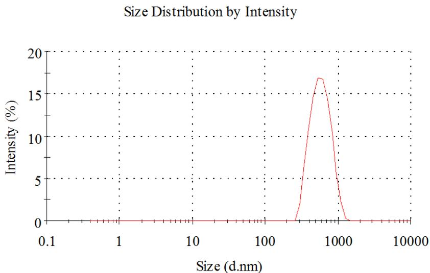
**Fig. 5.** Particle size distribution of crosslinking starch adhesive
