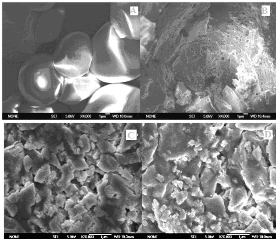
**Fig. 3.** SEM graphs of starch and paper surface: A and B are the SEM graph of cassava starch and crosslinked cassava starch, respectively; C and D are the SEM graph of the coated paper surface with the complex adhesive and SBR latex adhesive, respectively.
