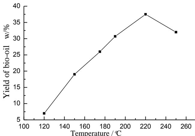
**Fig. 2.** Effect of pyrolytic temperature on the yield of bio-oil
