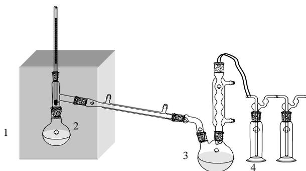
**Fig. 1.** Schematic layout of the pyrolysis experimental setup. 1) Microwave oven; 2) Reaction flask; 3) Receiving flask; 4) Gas-washing bottle
