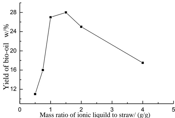
**Fig. 3.** Effect of mass ratio of IL to straw on bio-oil yield
