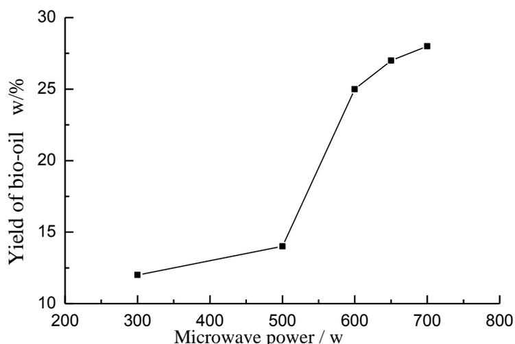
**Fig. 5.** Effect of microwave irradiation power on the yield of bio-oil
