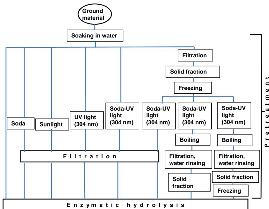
Pretreatment times: NaOH 30h, under artificial UV 30 h; sunlight 90 h; freezing 15 h; boiling 1 h; soaking in water 24 h
