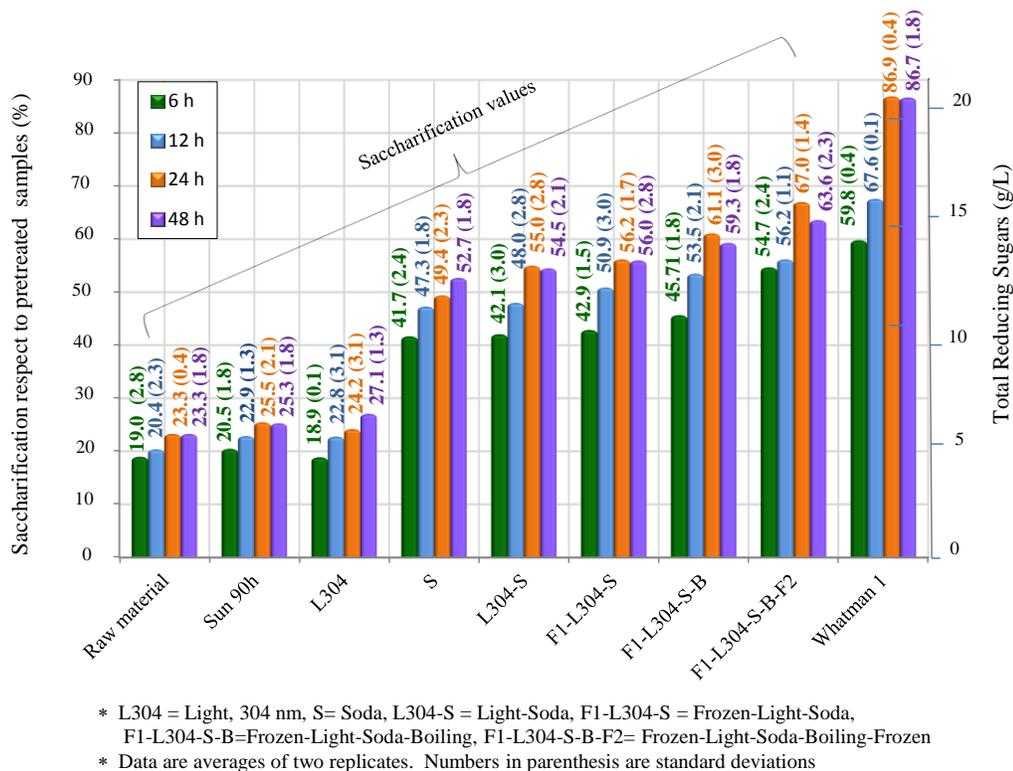
**Fig. 3.** Fermentable sugar yield of *L. rotundiflorus* hydrolysates obtained with different pretreatments, after distinct elapsed hydrolysis times. Total reducing sugars (g/L) concentration is read on the right axis, whereas saccharification (%) with respect to pretreated raw material is read on the left axis.
