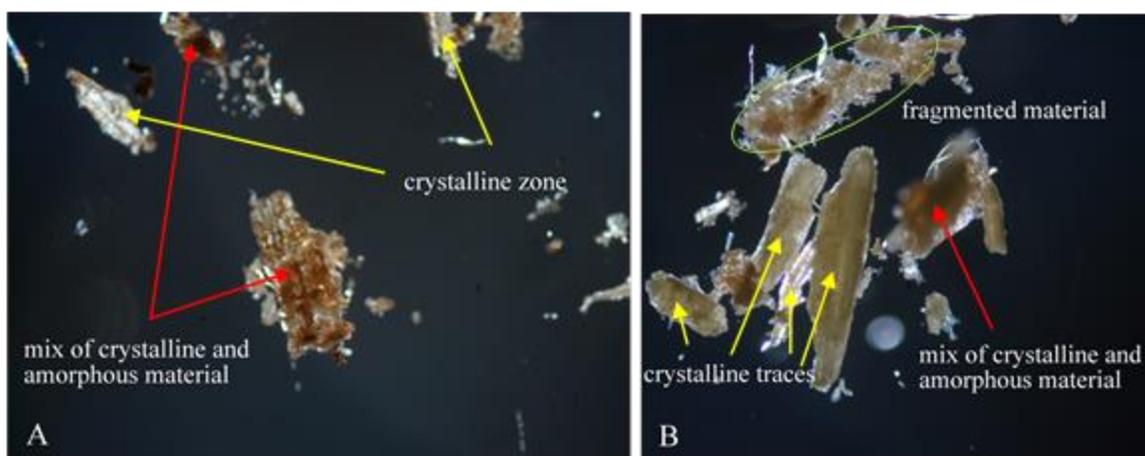
**Fig. 4.** Microphotographs under polarized light of *L. rotundiflorus* samples, 50X. A) L304 pretreatment and B) F1-L304-S-B-F2 pretreatment
