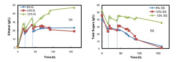
**Fig. 4.** Ethanol production and consumption of total sugars during SSF of different suspended solids. The dashed lines indicate the dilution effect created in the fermentor after each stepwise addition of pretreated birch slurry.
