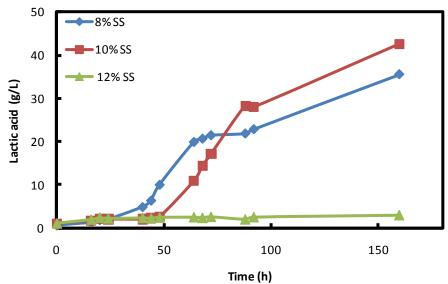
Fig. 1. Lactic acid production during SSF with different SS concentrations
