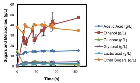
Fig. 2. Sugar and metabolite concentrations during SSF with 12% SS
