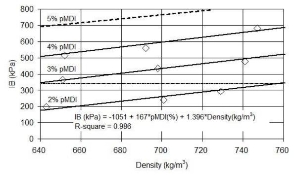
Fig. 5. The internal bond (IB) strength of oriented structural straw board as a function of resin content and panel density
