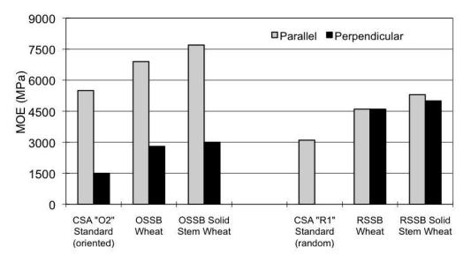
**Fig. 4.** Effects of straw species and strand orientation on panel stiffness (MOE). RSSB = random structural straw board
