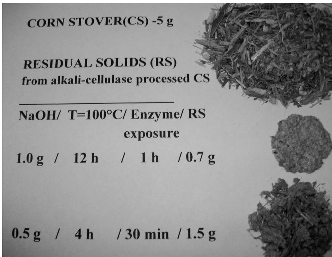
**Fig. 4.** 5 g corn stover before processing; residual solids resulting from Alkcell processing under two sets of conditions
