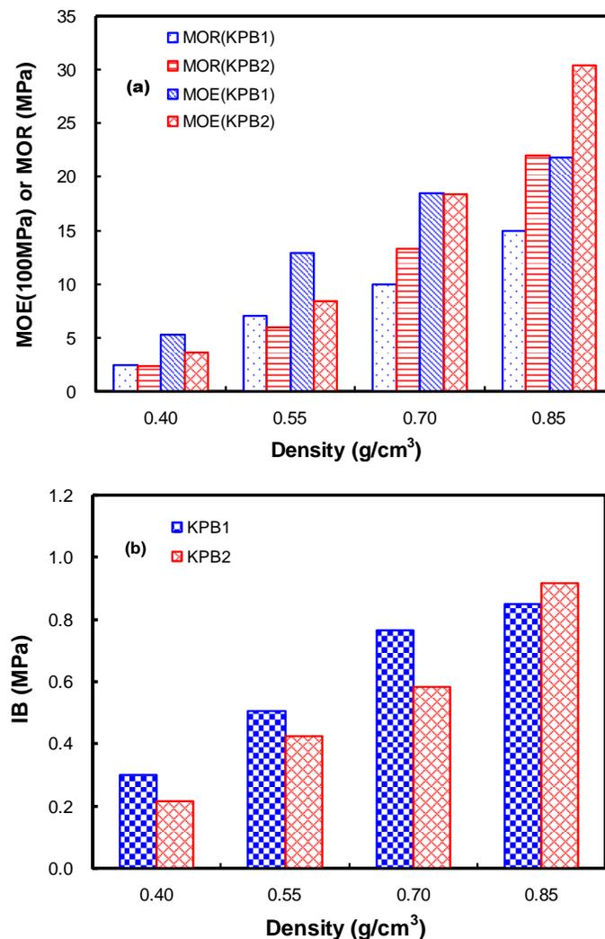
Fig. 2. Bending (a) and internal bond (b) properties of single-layer KPBI
