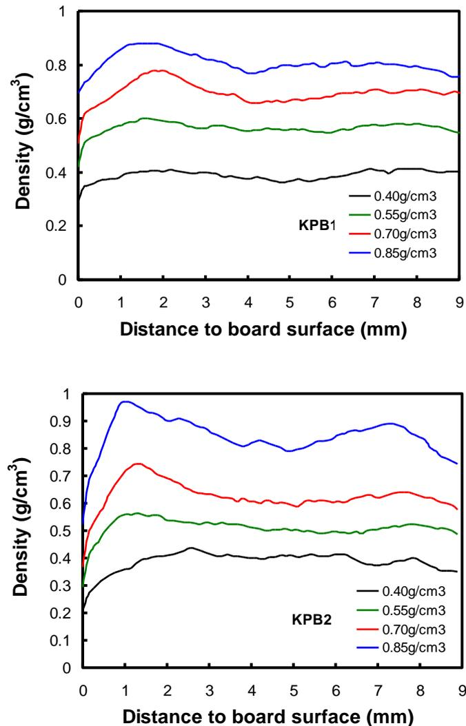
**Fig. 1.** Vertical density profile of single-layer KPBI
