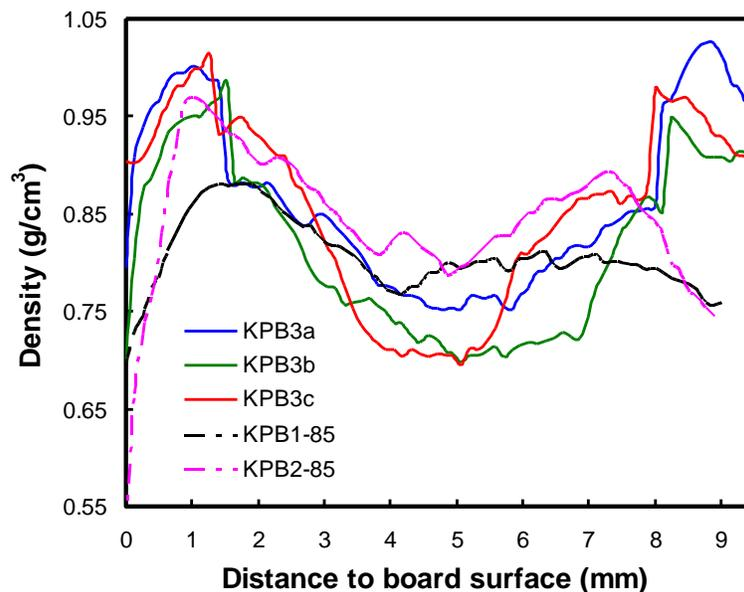
**Fig. 4.** Density profiles of three-layer KPBs
