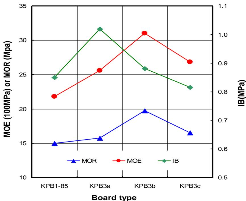
**Fig. 5.** Influences of construction on MOE, MOR, and IB strength
