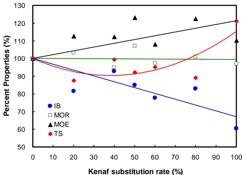
Fig. 6. Board performance variations with kenaf substitution rates
