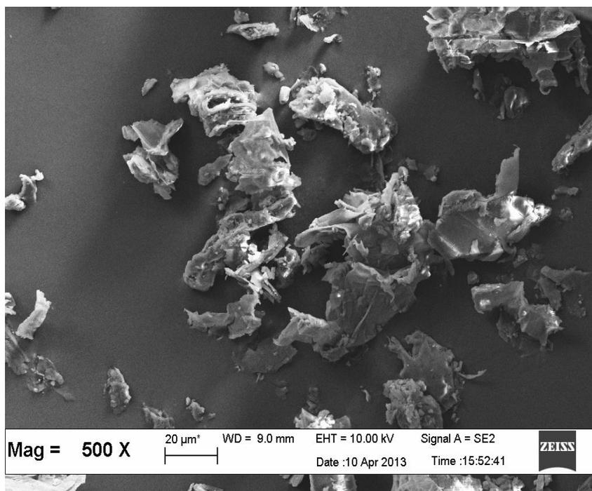
**Fig. 3.** SEM micrograph of the irregular morphology of peanut shell powder
