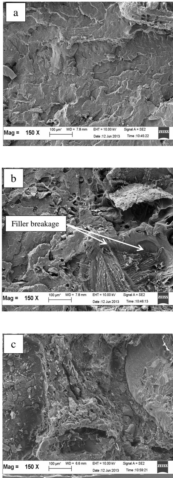
**Fig. 6.** SEM micrographs of compatibilized RPP/PSP composites at (a) 10%, (b) 20%, and (c) 40% (by weight) PSP loadings
