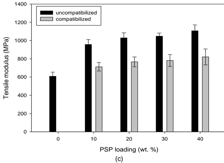
**Fig. 2.** (a) Tensile strength, (b) elongation at break, and (c) tensile modulus of RPP/PSP composites with and without compatibilizer at different PSP loadings
