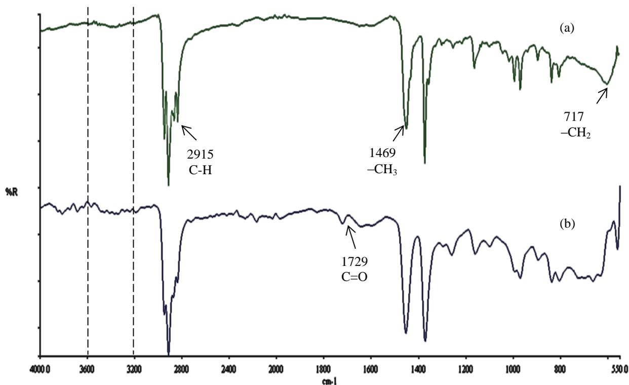
Fig. 4. IR spectra of RPP/PSP composites (a) uncompatibilized and (b) compatibilized with PEAA
