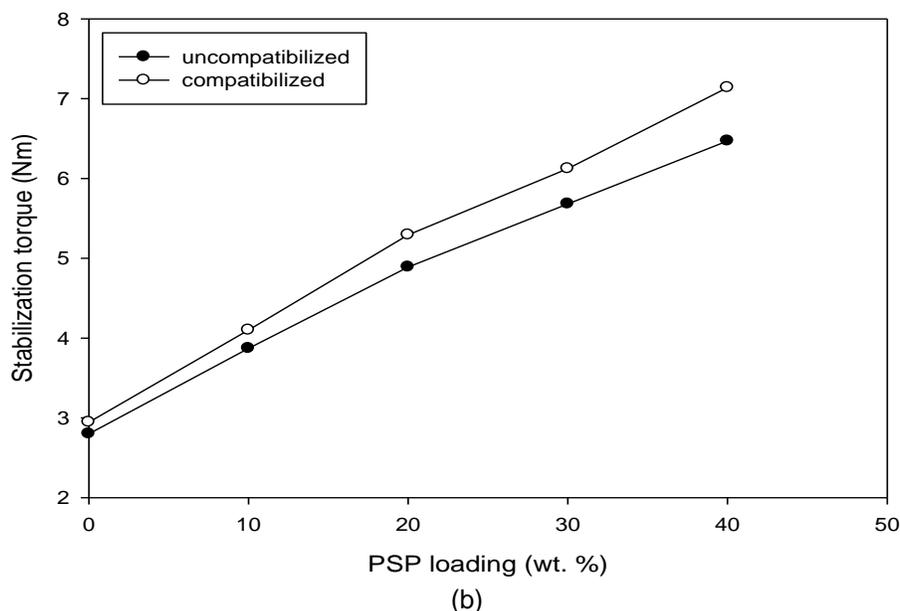
**Fig. 1. (a)** The processing torque of compatibilized RPP/PSP composites, and **(b)** the stabilization torque of RPP/PSP composites with and without compatibilizer at different PSP loadings
