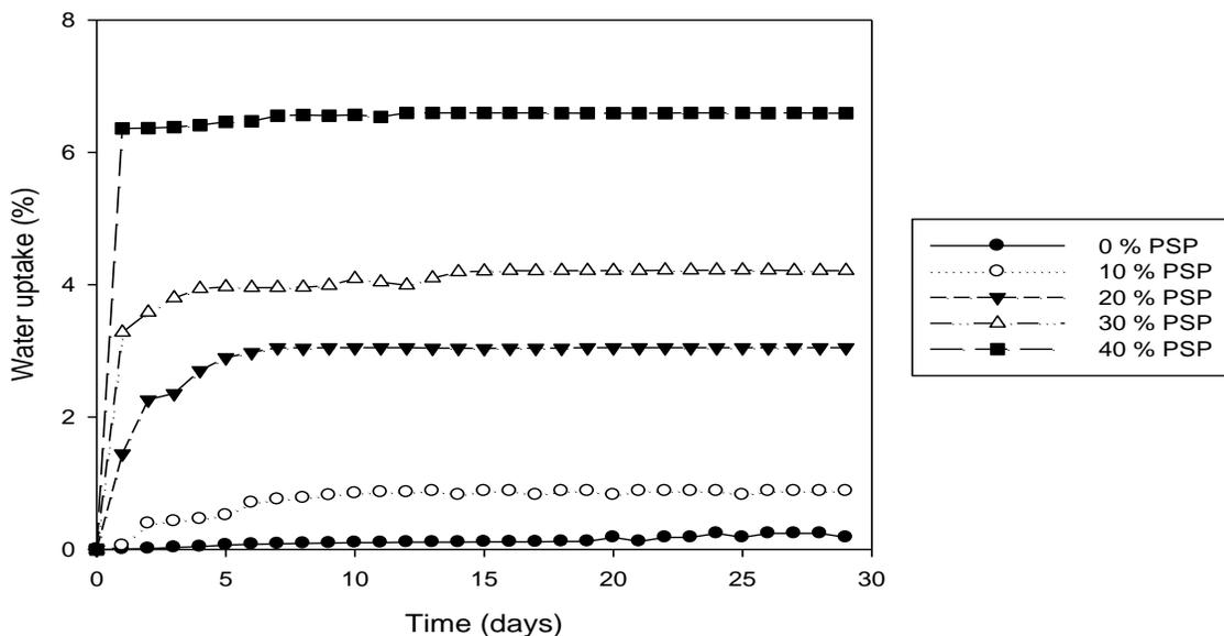
Fig. 7. Water uptake of uncompatibilized RPP/PSP composites at different PSP loadings
