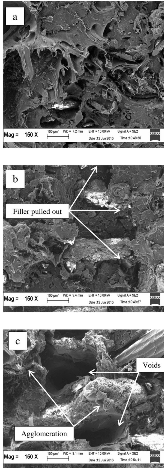
**Fig. 5.** SEM micrographs of uncompatibilized RPP/PSP composites at (a) 10%, (b) 20%, and (c) 40% (by weight) PSP loadings
