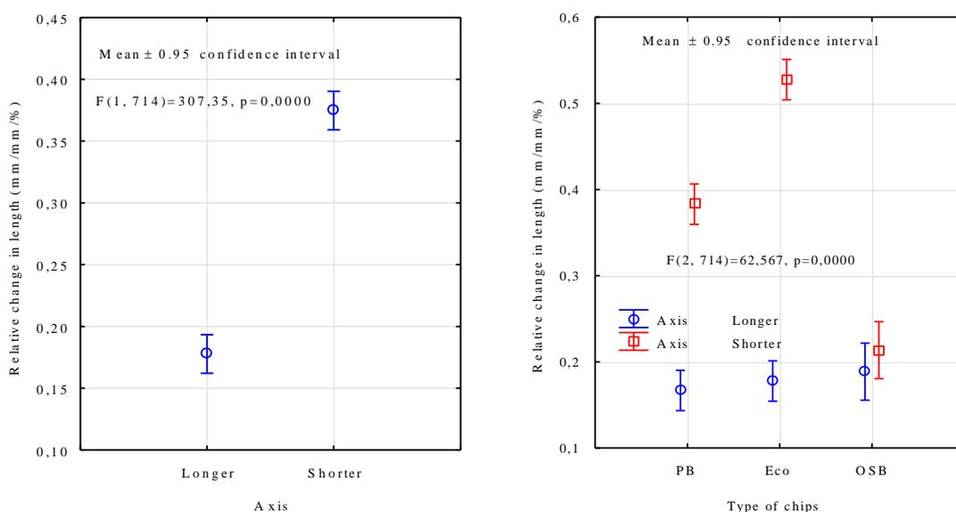
**Fig. 2.** Effect of the type of chips in the OSB core layer on the change in length triggered by changes in humidity; a) importance of the board axis, and b) relationship between the type of chips and the board axis
