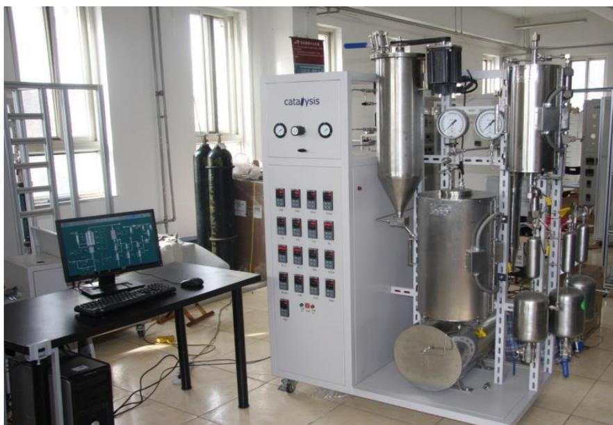
**Fig. 1.** The BJFU fluidized bed pyrolysis system. (a) Schematic diagram of the system. 1, biomass feeding system; 2, fluidized bed reactor; 3, cyclone separator; 4, char collector; 5, condensers; 6, bio-oil collector; 7, gas washer. (b) Picture of the whole system
