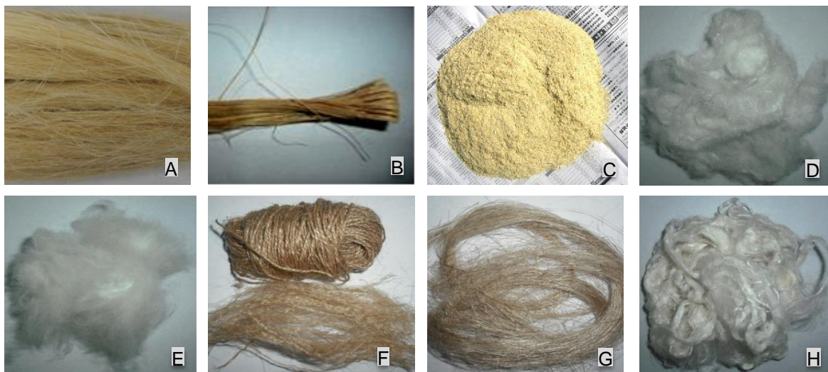
Fig. 1. Materials used in the tests. A: Natural bamboo fiber; B: Bamboo bundle; C: Bamboo powder; D: Regenerated bamboo fiber; E: Cotton fiber; F: Jute fiber; G: Flax fiber; H: Ramie fiber
